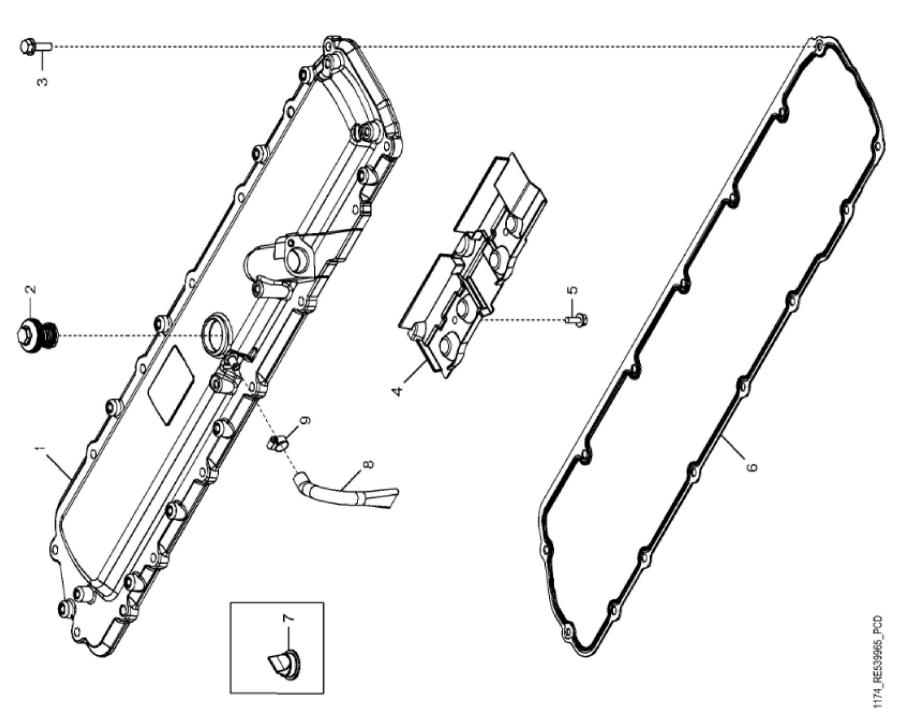
John Deere > Turf And Utility >TRACTOR >6230R - TRACTOR >6230R Tractor (Europe Edition, Engine SN: 6068UXXXXXXX)(Final Tier 4) >EN ENGINE 6068HL500-DZ104589 >EN00 ENGINE 6068HL500-DZ104589 6068HL500 >ST848860 - 1174 ROCKER ARM COVER
