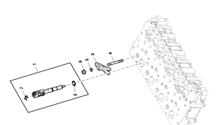
John Deere > Turf And Utility >TRACTOR >F5DFL413C - TRACTOR >5075GV Tractor (Engine F5D) IT4 (Europe Edition) >20 ENGINE >ST833621 - INJECTION NOZZLE
