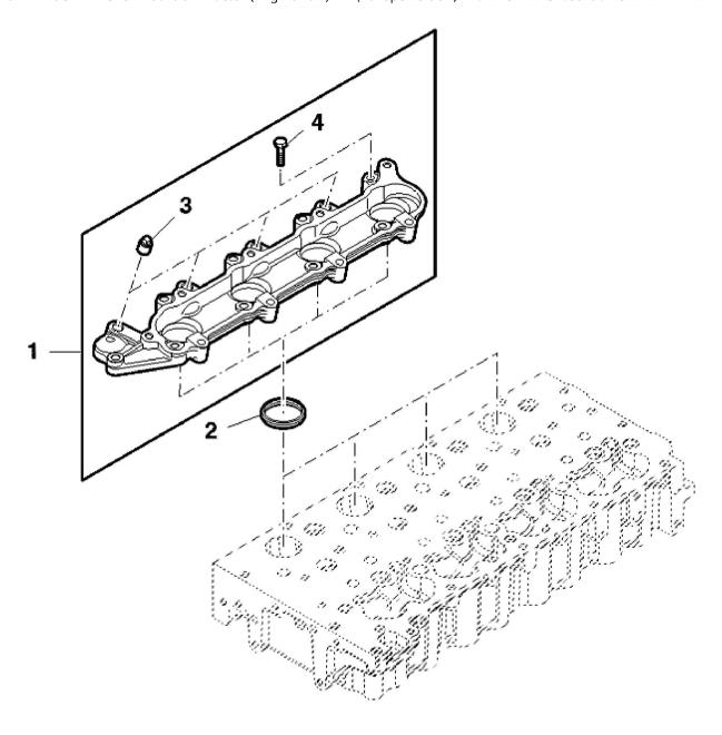
John Deere > Turf And Utility >TRACTOR >F5DFL413C - TRACTOR >5075GV Tractor (Engine F5D) IT4 (Europe Edition) >20 ENGINE >ST833498 - CYLINDER HEAD HOUSING
