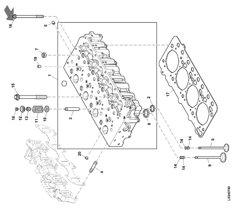
John Deere > Turf And Utility >TRACTOR >F5DFL413C - TRACTOR >5075GV Tractor (Engine F5D) IT4 (Europe Edition) >20 ENGINE >ST833491 - CYLINDER HEAD
