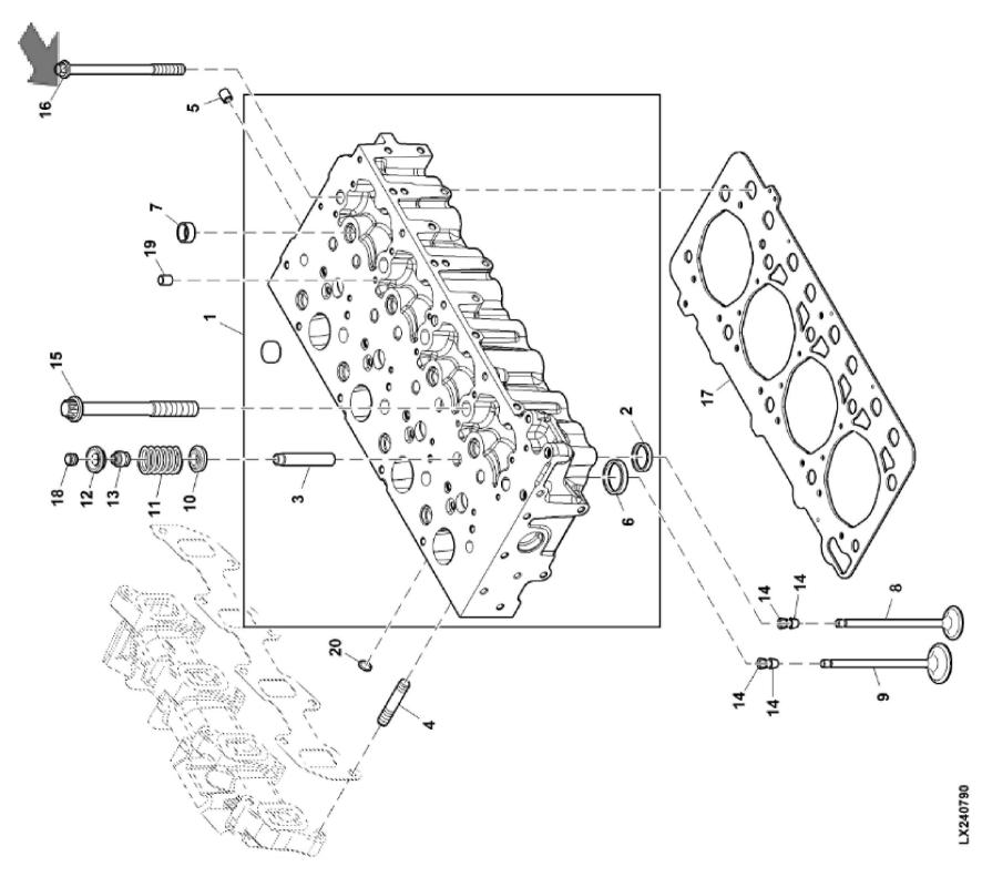
John Deere > Turf And Utility >TRACTOR >F5DFL413R - TRACTOR >5105GN Tractor (Engine F5D) IT4 (Europe Edition) >20 ENGINE >ST833491 - CYLINDER HEAD
