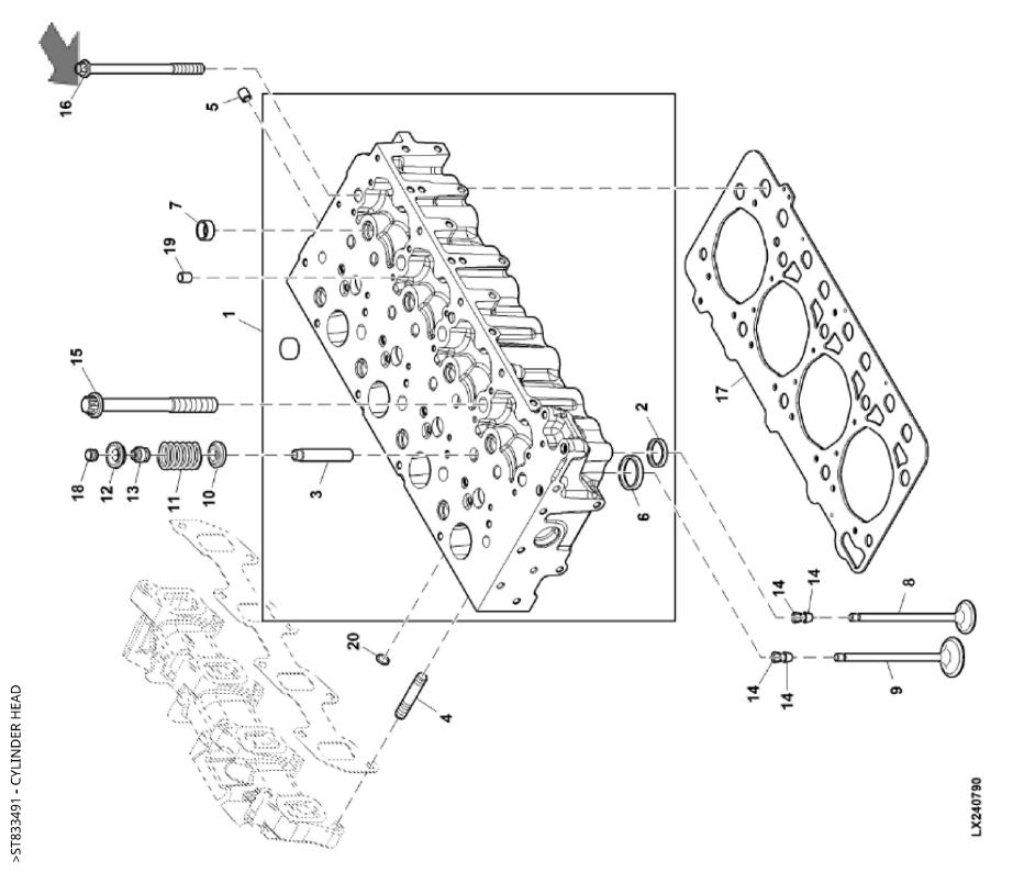
John Deere > Turf And Utility >TRACTOR >F5DFL413C - TRACTOR >5075GN Tractor (Engine F5D) IT4 (Europe Edition) >20 ENGINE >ST833491 - CYLINDER HEAD
