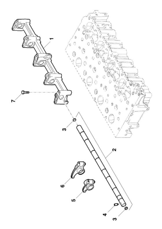
John Deere > Turf And Utility >TRACTOR >F5DFL413T - TRACTOR >5090GF Tractor (Engine F5D) IT4 (Europe Edition) >20 ENGINE >ST833506 - ROCKER ARM / SHAFT
