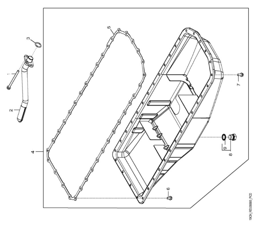
John Deere > Turf And Utility >TRACTOR >6175M - TRACTOR >6175M Tractor (Europe Edition, Engine SN: 6068GXXXXXX)(Tier 2)(S.N. 860524-) >EN ENGINE 6068HL289-DZ105553-ETN150959 >EN00 ENGINE 6068HL289-DZ105553-ETN150959 6068HL289 >ST711844 - 19CH OIL PAN
