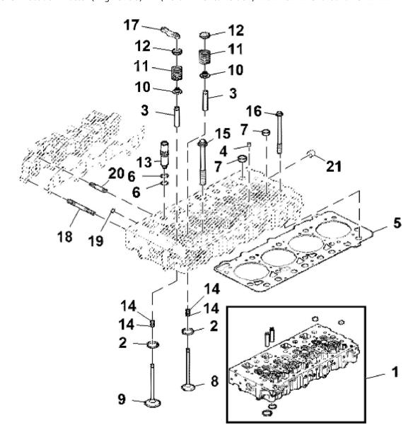
John Deere > Turf And Utility >TRACTOR >F5GFL413L - TRACTOR >5090GV Tractor (Engine F5G) FT4 (North America Edition) >20 ENGINE >ST845948 - CYLINDER HEAD
