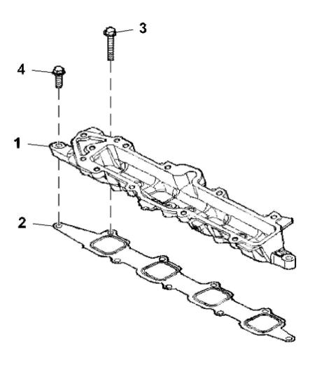
John Deere > Turf And Utility >TRACTOR >F5GFL413L - TRACTOR >5090GV Tractor (Engine F5G) FT4 (North America Edition) >20 ENGINE >ST845946 - AIR INTAKE MANIFOLD
