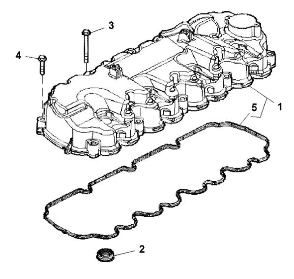
John Deere > Turf And Utility >TRACTOR >F5GFL413L - TRACTOR >5090GV Tractor (Engine F5G) FT4 (North America Edition) >20 ENGINE >ST845951 - CYLINDER HEAD COVER
