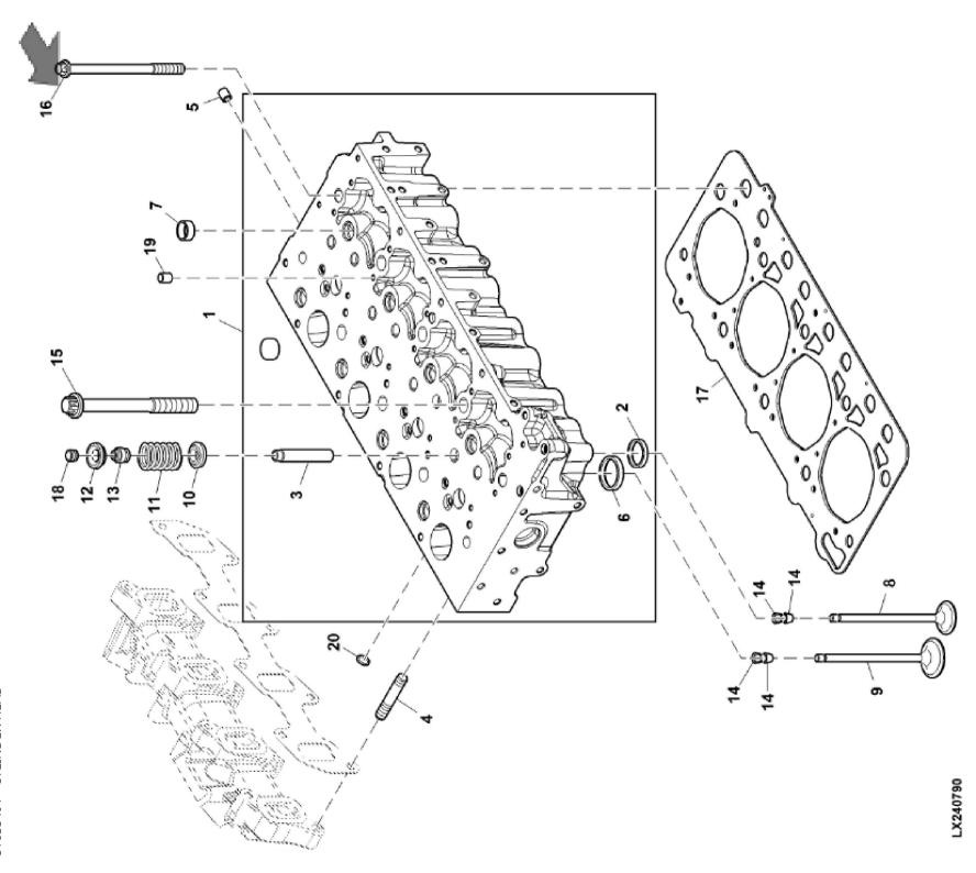
John Deere > Turf And Utility >TRACTOR >F5DFL413C - TRACTOR >5075GV Tractor (Engine F5D) FT4 (North America Edition) >20 ENGINE >ST833491 - CYLINDER HEAD
