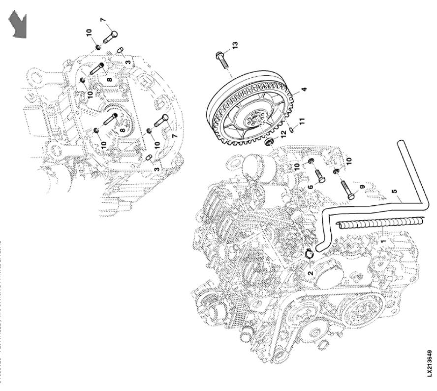
John Deere > Turf And Utility >TRACTOR >F5DFL413C - TRACTOR >5075GV Tractor (Engine F5D) FT4 (North America Edition) >20 ENGINE >ST833025 - FLYWHEEL / MOUNTING PARTS, ENGINE
