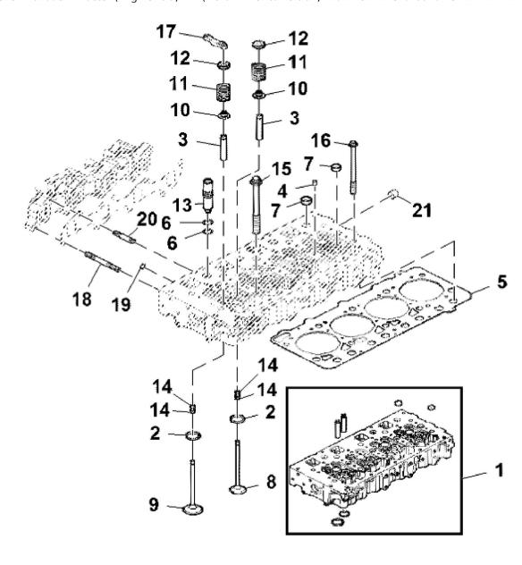
John Deere > Turf And Utility >TRACTOR >F5GFL413J - TRACTOR >5100GN Tractor (Engine F5G) FT4 (North America Edition) >20 ENGINE >ST845948 - CYLINDER HEAD
