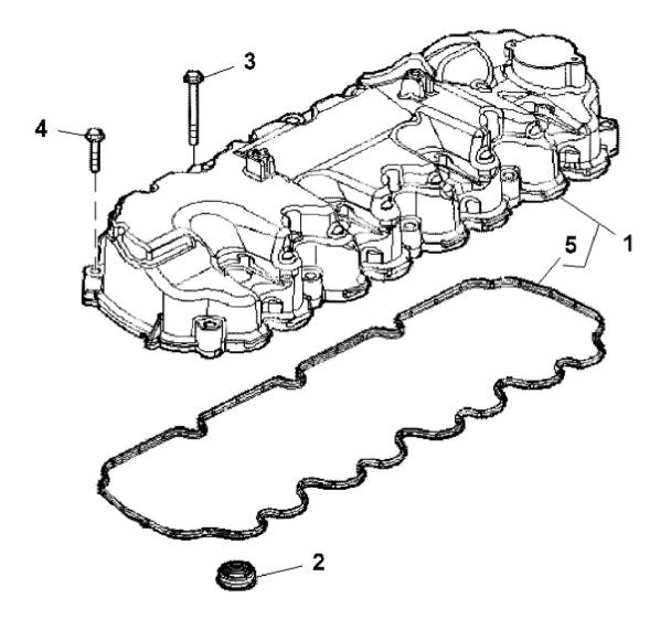
John Deere > Turf And Utility >TRACTOR >F5GFL413J - TRACTOR >5100GN Tractor (Engine F5G) FT4 (North America Edition) >20 ENGINE >ST845951 - CYLINDER HEAD COVER
