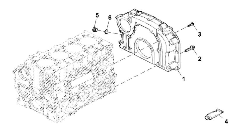
John Deere > Turf And Utility >TRACTOR >F5GFL413J - TRACTOR >5100GN Tractor (Engine F5G) FT4 (North America Edition) >20 ENGINE >ST845945 - FLYWHEEL HOUSING
