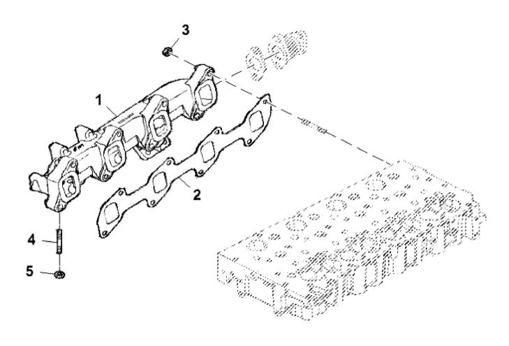
John Deere > Turf And Utility >TRACTOR >F5GFL413J - TRACTOR >5100GN Tractor (Engine F5G) FT4 (North America Edition) >20 ENGINE >ST845942 - EXHAUST MANIFOLD
