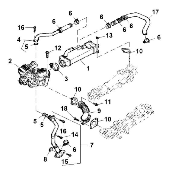
John Deere > Turf And Utility >TRACTOR >F5GFL413J - TRACTOR >5100GN Tractor (Engine F5G) FT4 (North America Edition) >20 ENGINE >ST845952 - EXHAUST GAS RECIRCULATION
