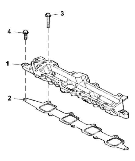
John Deere > Turf And Utility >TRACTOR >F5GFL413J - TRACTOR >5100GN Tractor (Engine F5G) FT4 (North America Edition) >20 ENGINE >ST845946 - AIR INTAKE MANIFOLD
