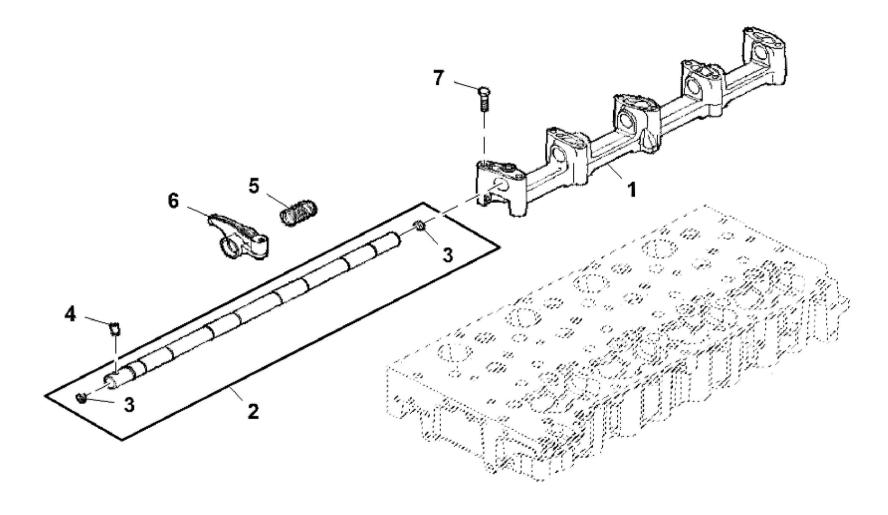
John Deere > Turf And Utility >TRACTOR >F5GFL413J - TRACTOR >5100GN Tractor (Engine F5G) FT4 (North America Edition) >20 ENGINE >ST845947 - ROCKER ARM / SHAFT
