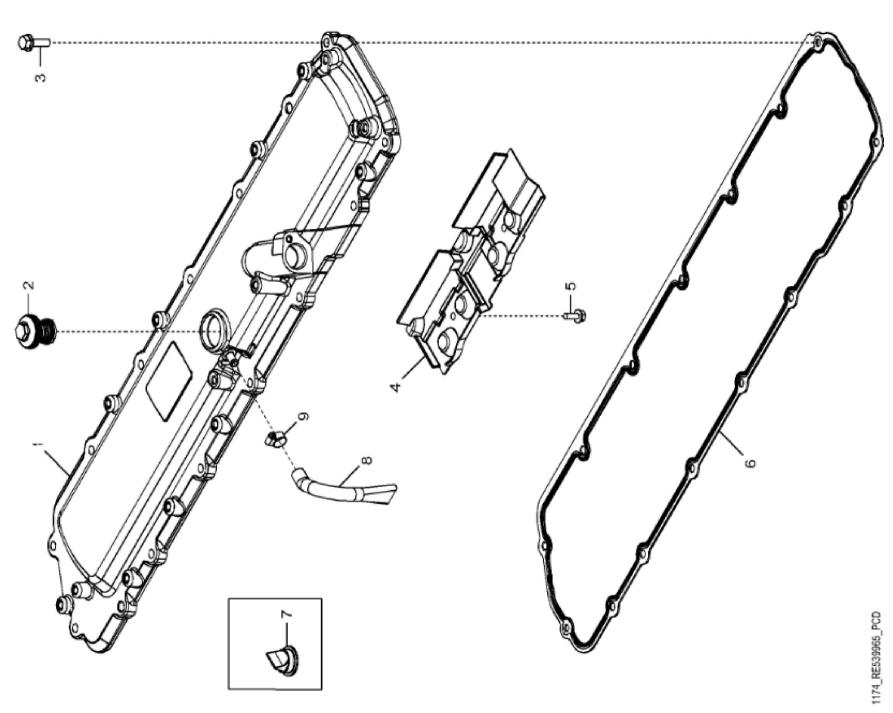
John Deere > Turf And Utility >TRACTOR >6195M - TRACTOR >6195M Tractor (North America Edition, Engine SN: 6068UXXXXXXX)(Final Tier 4) >E1 ENGINE 6068HL502-DZ10433-ETN131690 >E100 ENGINE 6068HL502-DZ10433-ETN131690 6068HL502 >ST164694 - 1174 ROCKER ARM COVER
