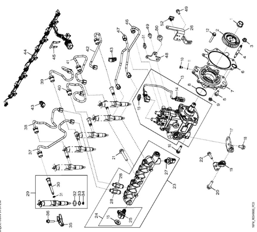
John Deere > Turf And Utility >TRACTOR >6195M - TRACTOR >6195M Tractor (North America Edition, Engine SN: 6068UXXXXXXX)(Final Tier 4) >E1 ENGINE 6068HL502-DZ10433-ETN131690 >E100 ENGINE 6068HL502-DZ10433-ETN131690 6068HL502 >ST751293 - 16FM FUEL INJECTION SYSTEM
