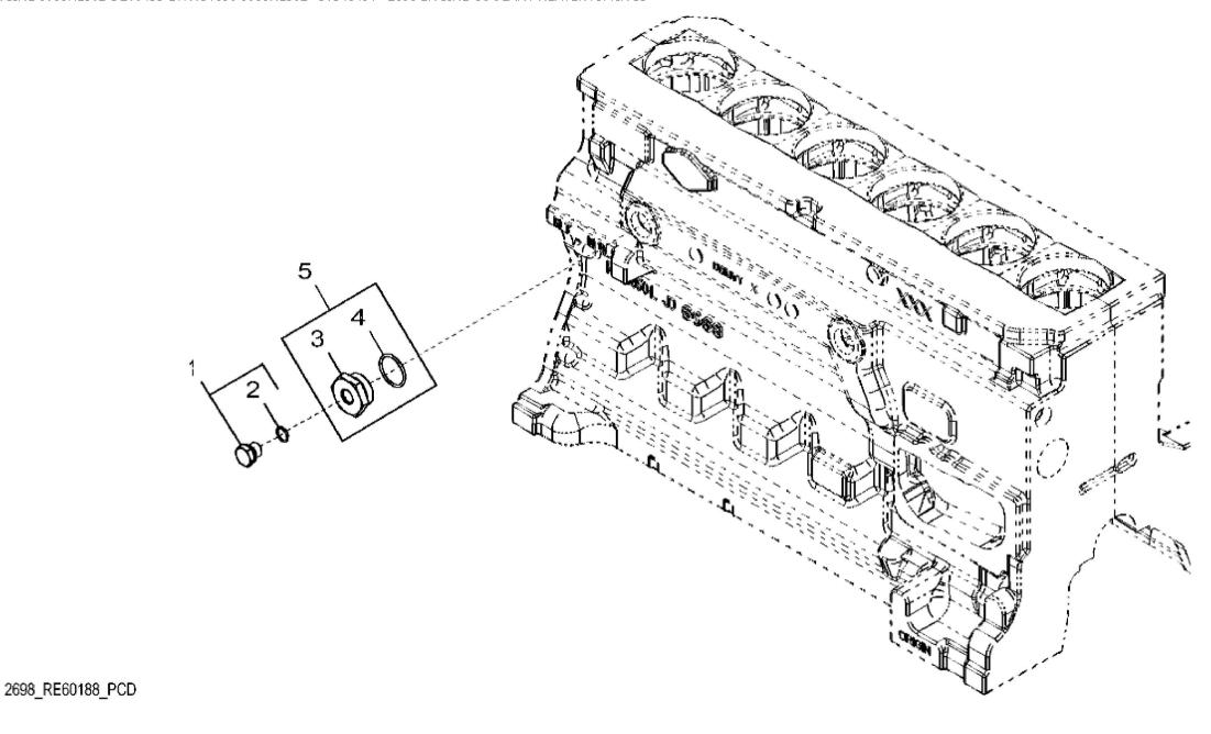
John Deere > Turf And Utility >TRACTOR >6195M - TRACTOR >6195M Tractor (North America Edition, Engine SN: 6068UXXXXXX)(Final Tier 4) >E1 ENGINE 6068HL502-DZ10433-ETN131690 >E100 ENGINE 6068HL502-DZ10433-ETN131690 6068HL502 >ST348491 - 2698 ENGINE COOLANT HEATER FITTINGS
