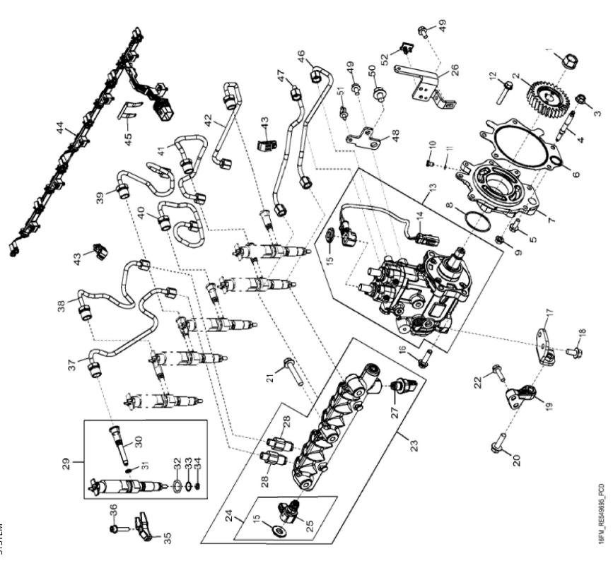
John Deere > Turf And Utility >TRACTOR >6195M - TRACTOR >6195M Tractor (Europe Edition, Engine SN: 6068UXXXXXX)(Final Tier 4) >E1 ENGINE 6068HL502-DZ10433-ETN131690 >E100 ENGINE 6068HL502-DZ10433-ETN131690 6068HL502 >ST751293 - 16FM FUEL INJECTION SYSTEM
