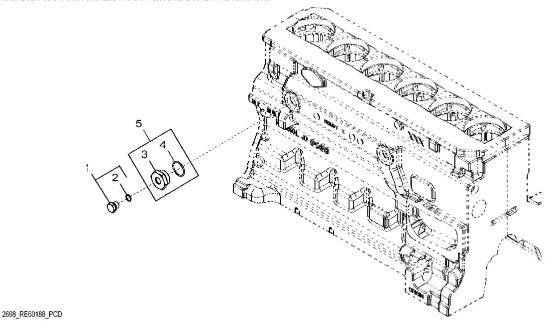
John Deere > Turf And Utility >TRACTOR >6195M - TRACTOR >6195M Tractor (Europe Edition, Engine SN: 6068UXXXXXX)(Final Tier 4) >E1 ENGINE 6068HL502-DZ10433-ETN131690 >E100 ENGINE 6068HL502-DZ10433-ETN131690 6068HL502 >ST348491 - 2698 ENGINE COOLANT HEATER FITTINGS
