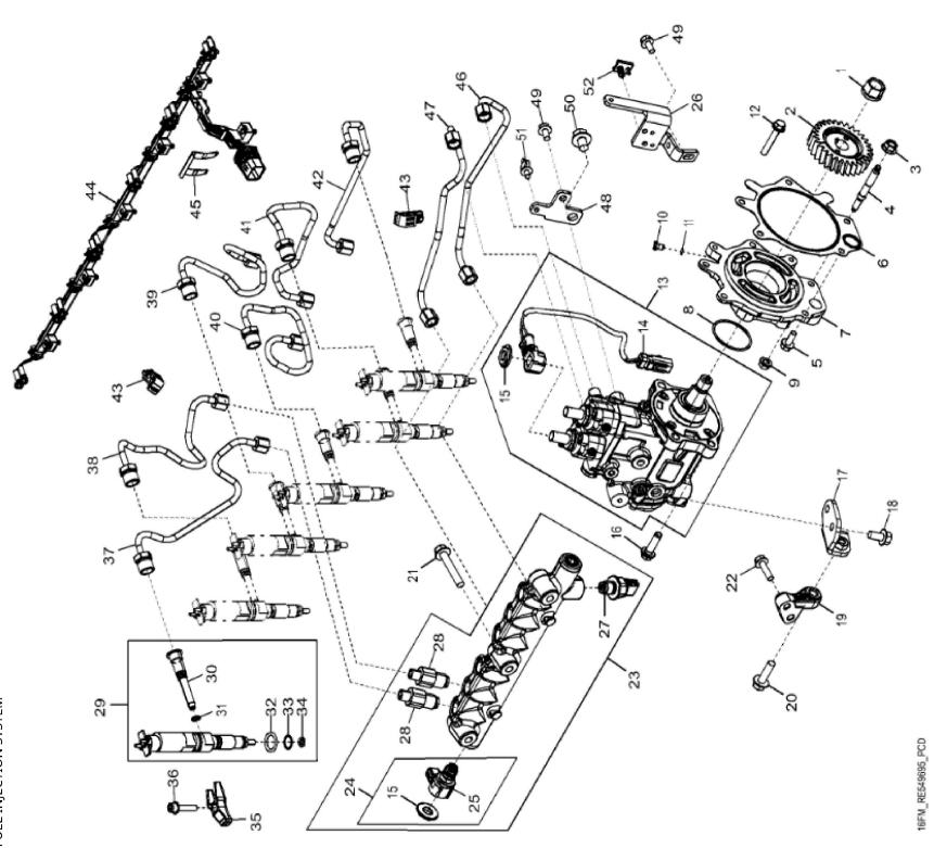
John Deere > Turf And Utility >TRACTOR >6175M - TRACTOR >6175M Tractor (Europe Edition, Engine SN: 6068UXXXXXX)(Final Tier 4) >E1 DIESEL ENGINE 6068HL498-DZ101710-ETN131689 >E100 DIESEL ENGINE 6068HL498-DZ101710-ETN131689 6068HL498 >ST751293 - 16FM FUEL INJECTION SYSTEM
