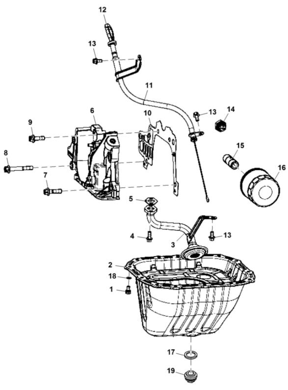
John Deere > Turf And Utility > UTILITY VEHICLE > XUV590i - UTILITY VEHICLE > XUV590i Gator Utility Vehicle > 20 ENGINE MM18178 > ST846159 - LUBRICATION SYSTEM
