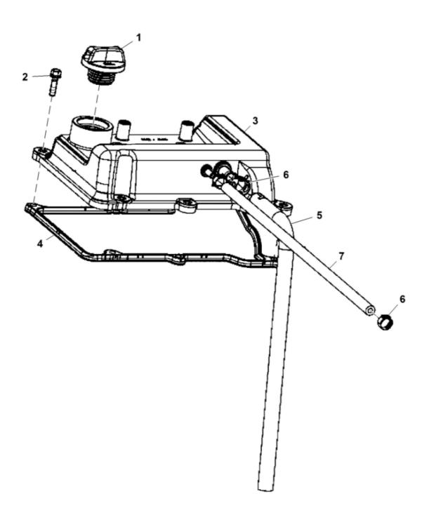
John Deere > Turf And Utility > UTILITY VEHICLE > XUV590i - UTILITY VEHICLE > XUV590i Gator Utility Vehicle > 20 ENGINE MM18178 > ST846119 - CRANKCASE VENTILATION SYSTEM
