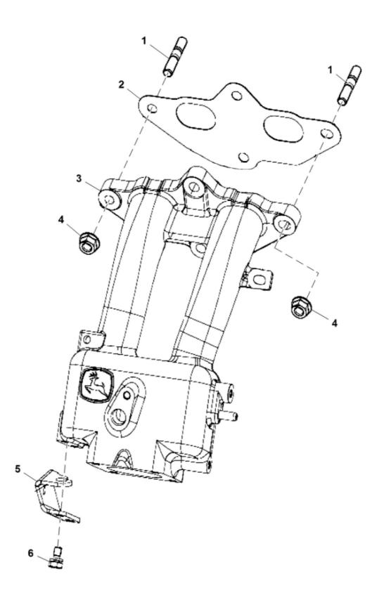
John Deere > Turf And Utility > UTILITY VEHICLE > XUV590i - UTILITY VEHICLE > XUV590i Gator Utility Vehicle > 20 ENGINE MM18178 > ST846095 - INTAKE MANIFOLD ASSEMBLY
