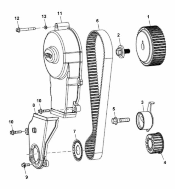
John Deere > Turf And Utility > UTILITY VEHICLE > XUV590i - UTILITY VEHICLE > XUV590i Gator Utility Vehicle > 20 ENGINE MM18178 > ST846181 - TIMING DRIVE
