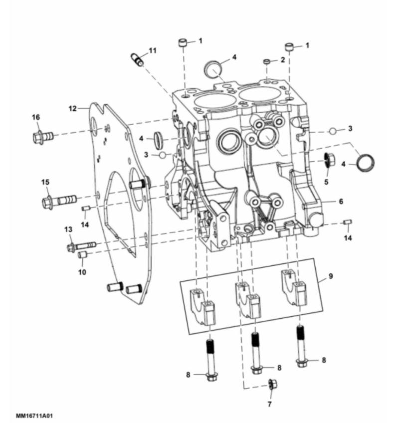
John Deere > Turf And Utility > UTILITY VEHICLE > XUV590i - UTILITY VEHICLE > XUV590i Gator Utility Vehicle > 20 ENGINE MM18178 > ST846079 - CYLINDER BLOCK
