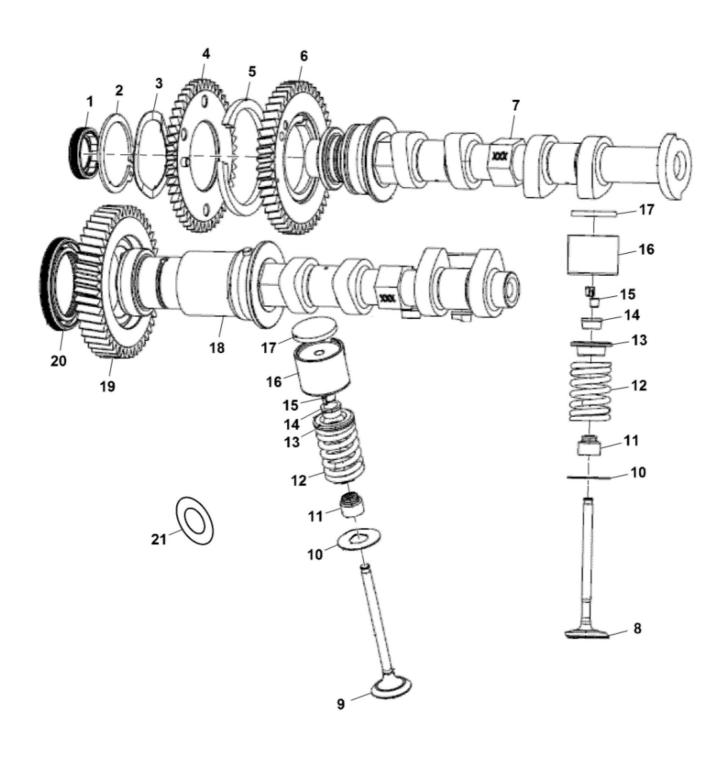
John Deere > Turf And Utility > UTILITY VEHICLE > XUV590i - UTILITY VEHICLE > XUV590i Gator Utility Vehicle > 20 ENGINE MM18178 > ST845931 - VALVE TRAIN
