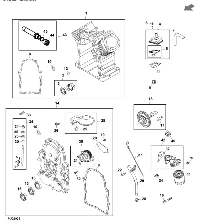
John Deere > Turf And Utility > UTILITY VEHICLE > XUV560 S4 - UTILITY VEHICLE > XUV560 S4 Gator Utility Vehicle > 20 ENGINE MM17462 > ST863635 - CRANKCASE
