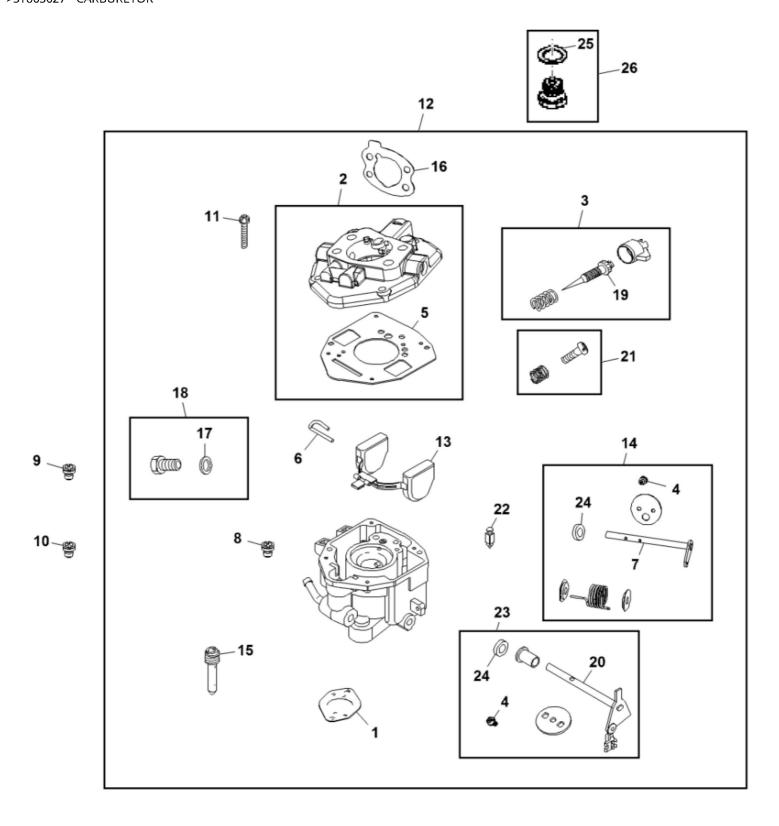
John Deere > Turf And Utility > UTILITY VEHICLE > XUV560 S4 - UTILITY VEHICLE > XUV560 S4 Gator Utility Vehicle > 30 FUEL AND AIR > ST863627 - CARBURETOR
