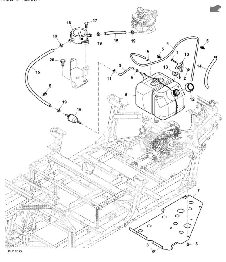
John Deere > Turf And Utility > UTILITY VEHICLE > XUV560 S4 - UTILITY VEHICLE > XUV560 S4 Gator Utility Vehicle > 30 FUEL AND AIR > ST845145 - FUEL TANK
