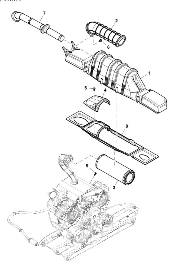
John Deere > Turf And Utility > UTILITY VEHICLE > XUV560 S4 - UTILITY VEHICLE > XUV560 S4 Gator Utility Vehicle > 30 FUEL AND AIR > ST845147 - INTAKE SYSTEM
