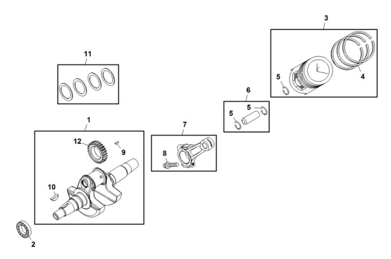
John Deere > Turf And Utility > UTILITY VEHICLE > XUV560 S4 - UTILITY VEHICLE > XUV560 S4 Gator Utility Vehicle > 20 ENGINE MM17462 > ST863631 - CRANK SHAFT AND PISTON
