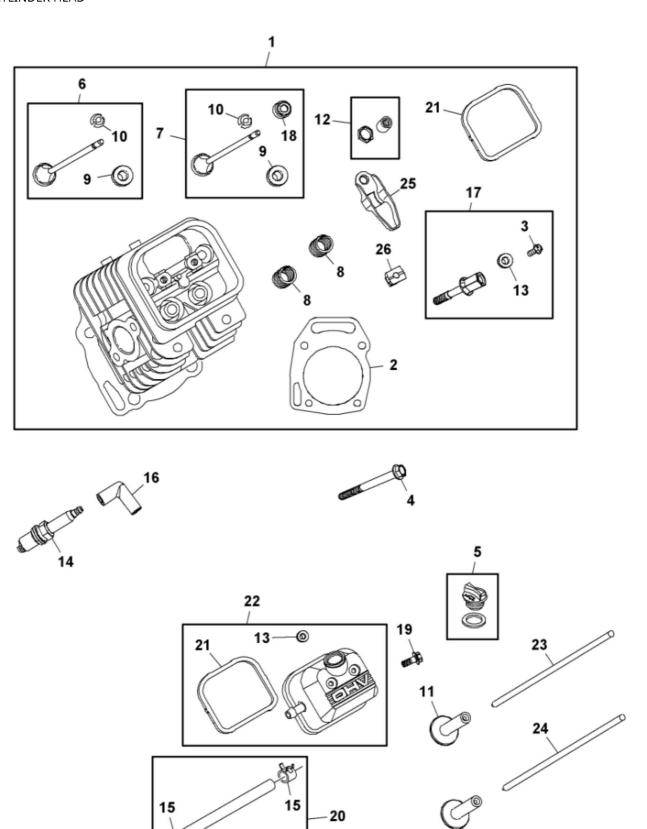
John Deere > Turf And Utility > UTILITY VEHICLE > XUV560 - UTILITY VEHICLE > XUV560 Gator Utility Vehicle > 20 ENGINE MM17462 > ST863638 - CYLINDER HEAD
