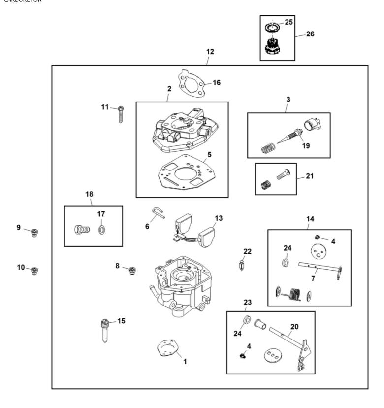
John Deere > Turf And Utility > UTILITY VEHICLE > XUV560 - UTILITY VEHICLE > XUV560 Gator Utility Vehicle > 30 FUEL AND AIR > ST863627 - CARBURETOR
