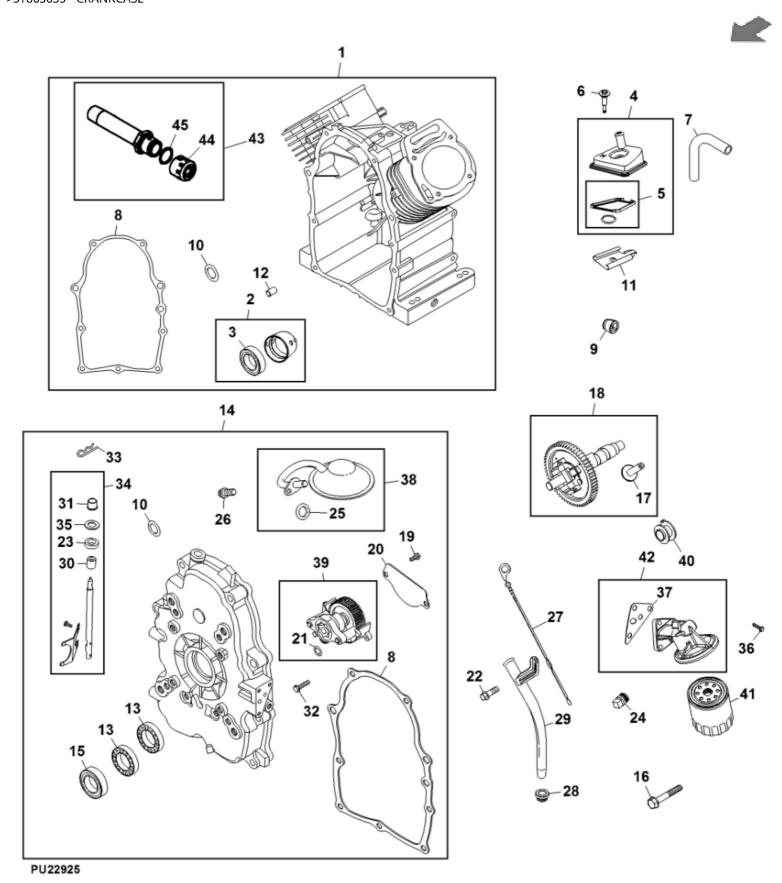
John Deere > Turf And Utility > UTILITY VEHICLE > XUV560 - UTILITY VEHICLE > XUV560 Gator Utility Vehicle > 20 ENGINE MM17462 > ST863635 - CRANKCASE
