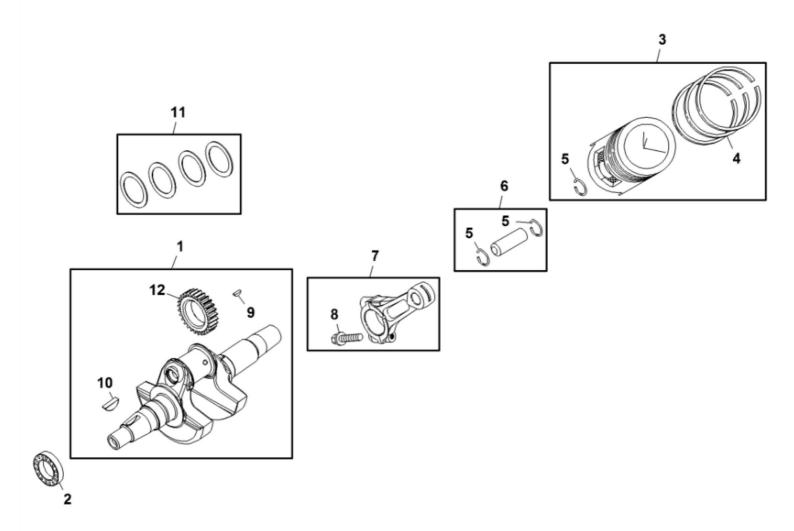
John Deere > Turf And Utility > UTILITY VEHICLE > XUV560 - UTILITY VEHICLE > XUV560 Gator Utility Vehicle > 20 ENGINE MM17462 > ST863631 - CRANK SHAFT AND PISTON
