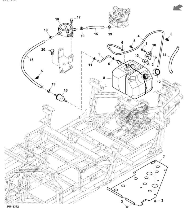
John Deere > Turf And Utility > UTILITY VEHICLE > XUV560 - UTILITY VEHICLE > XUV560 Gator Utility Vehicle > 30 FUEL AND AIR > ST845145 - FUEL TANK
