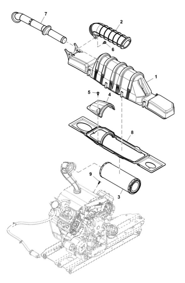
John Deere > Turf And Utility > UTILITY VEHICLE > XUV560 - UTILITY VEHICLE > XUV560 Gator Utility Vehicle > 30 FUEL AND AIR > ST845147 - INTAKE SYSTEM
