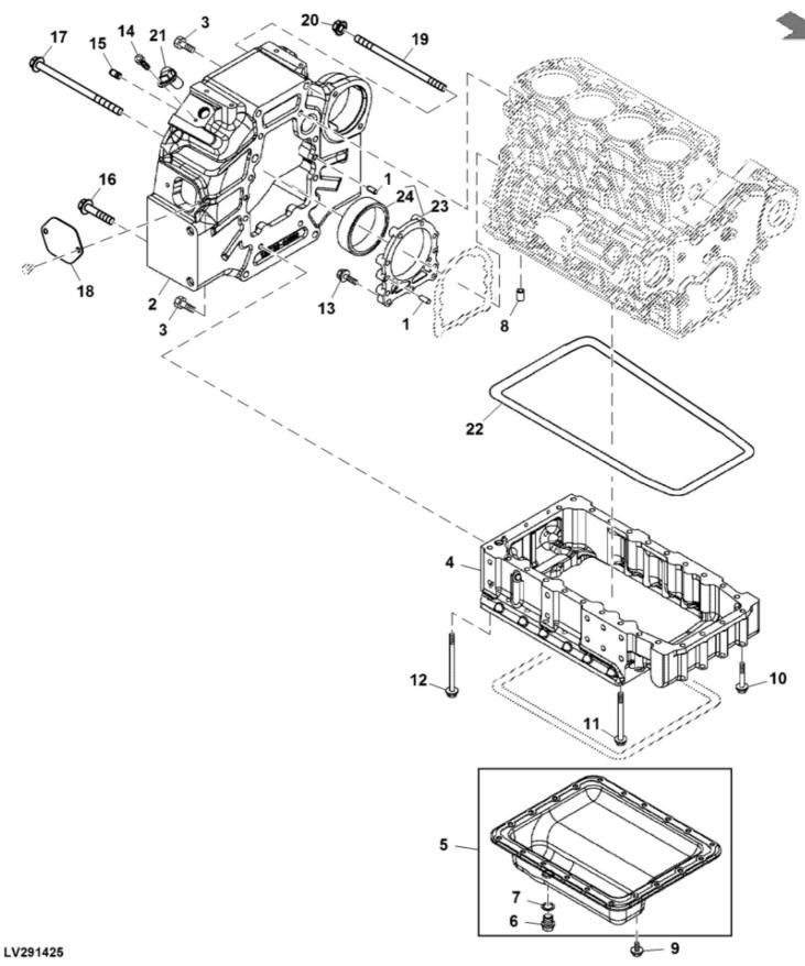
John Deere > Turf And Utility >TRACTOR, COMPACT UTILITY >4TNV86CT - TRACTOR, COMPACT UTILITY >4052R Compact Utility Tractor >20 ENGINE >ST770323 - FLYWHEEL HOUSING AND OIL SUMP
