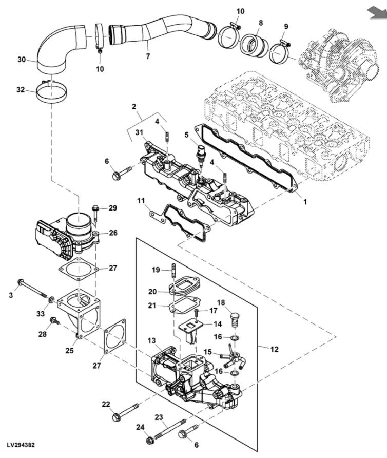
John Deere > Turf And Utility >TRACTOR, COMPACT UTILITY >4TNV86CT - TRACTOR, COMPACT UTILITY >4052R Compact Utility Tractor >20 ENGINE >ST770891 - SUCTION MANIFOLD
