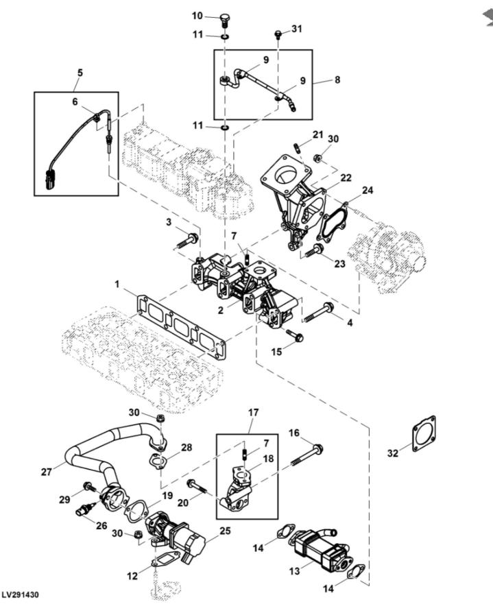
John Deere > Turf And Utility >TRACTOR, COMPACT UTILITY >4TNV86CT - TRACTOR, COMPACT UTILITY >4052R Compact Utility Tractor >20 ENGINE >ST770903 - EXHAUST MANIFOLD
