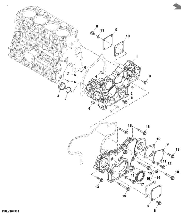
John Deere > Turf And Utility >TRACTOR, COMPACT UTILITY >4TNV86CT - TRACTOR, COMPACT UTILITY >4052R Compact Utility Tractor >20 ENGINE >ST770287 - GEAR HOUSING
