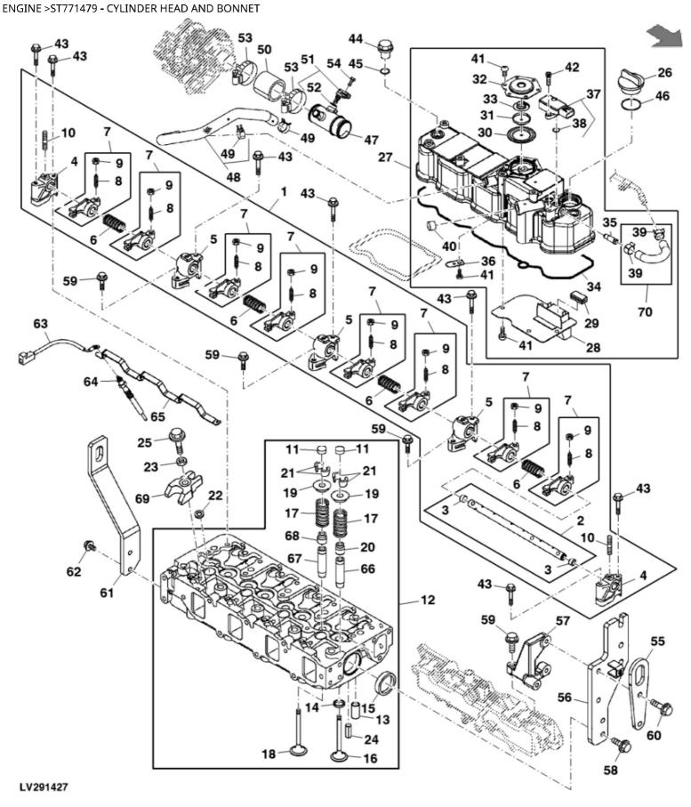
John Deere > Turf And Utility >TRACTOR, COMPACT UTILITY >4TNV86CT - TRACTOR, COMPACT UTILITY >4052M Compact Utility Tractor >20 ENGINE >ST771479 - CYLINDER HEAD AND BONNET
