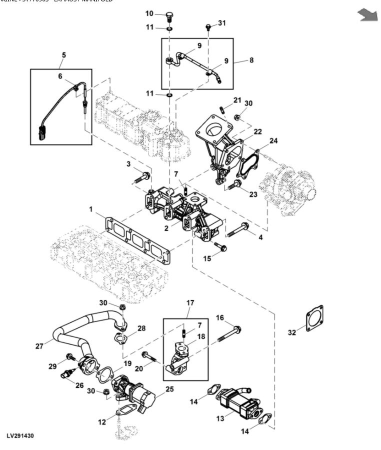
John Deere > Turf And Utility >TRACTOR, COMPACT UTILITY >4TNV86CT - TRACTOR, COMPACT UTILITY >4052M Compact Utility Tractor >20 ENGINE >ST770903 - EXHAUST MANIFOLD
