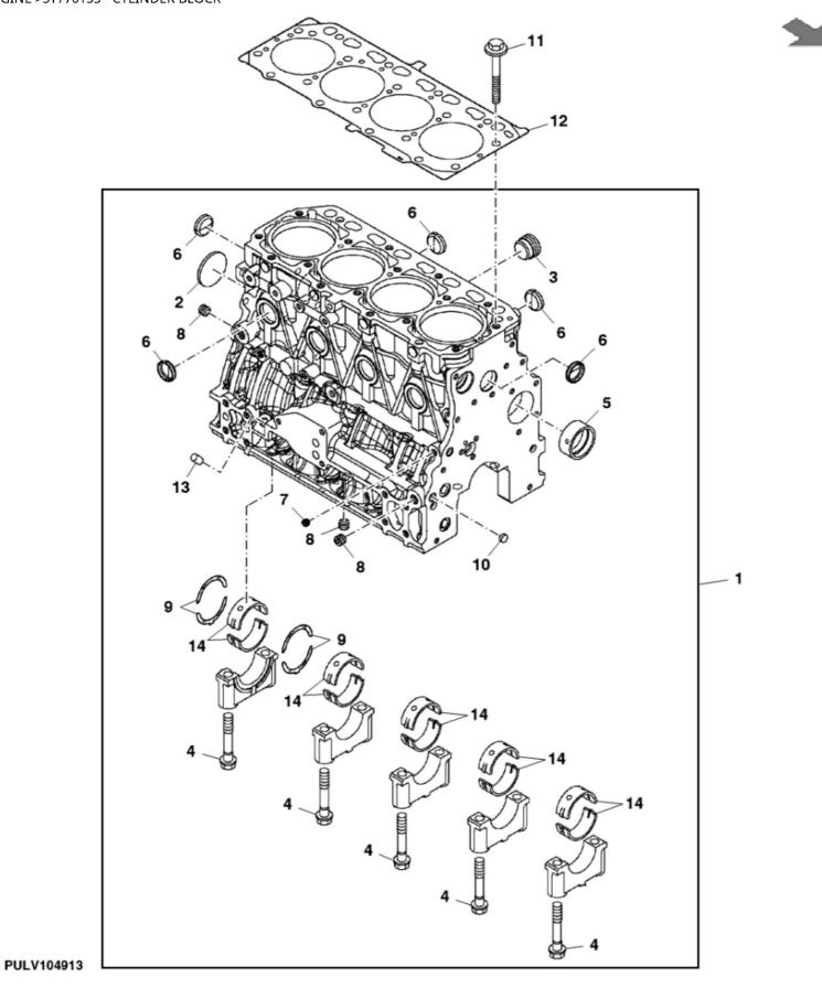
John Deere > Turf And Utility >TRACTOR, COMPACT UTILITY >4TNV86CT - TRACTOR, COMPACT UTILITY >4052M Compact Utility Tractor >20 ENGINE >ST770155 - CYLINDER BLOCK
