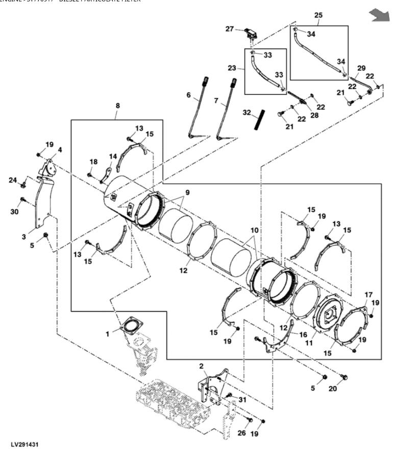
John Deere > Turf And Utility >TRACTOR, COMPACT UTILITY >4TNV86CT - TRACTOR, COMPACT UTILITY >4052M Compact Utility Tractor >20 ENGINE >ST770917 - DIESEL PARTICULATE FILTER
