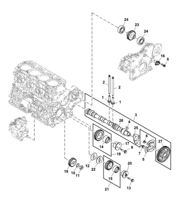
John Deere > Turf And Utility >TRACTOR, COMPACT UTILITY >4TNV86CT - TRACTOR, COMPACT UTILITY >4052M Compact Utility Tractor >20 ENGINE >ST770930 - CAMSHAFT AND DRIVING GEAR
