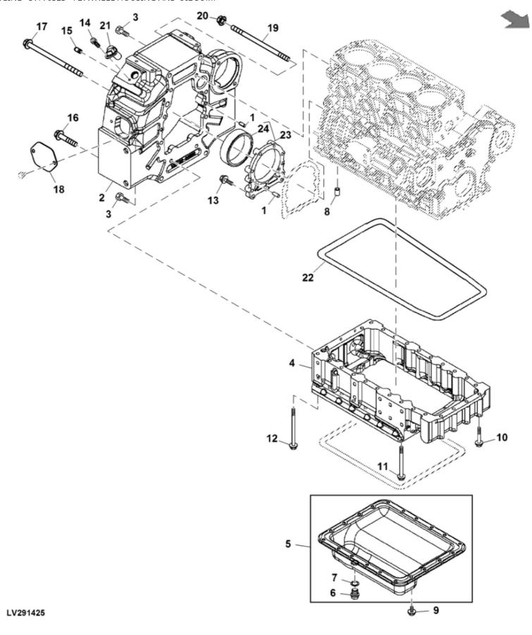
John Deere > Turf And Utility > TRACTOR, COMPACT UTILITY > 4TNV86CT - TRACTOR, COMPACT UTILITY > 4052M Compact Utility Tractor > 20 ENGINE > 5T770323 - FLYWHEEL HOUSING AND OIL SUMP
