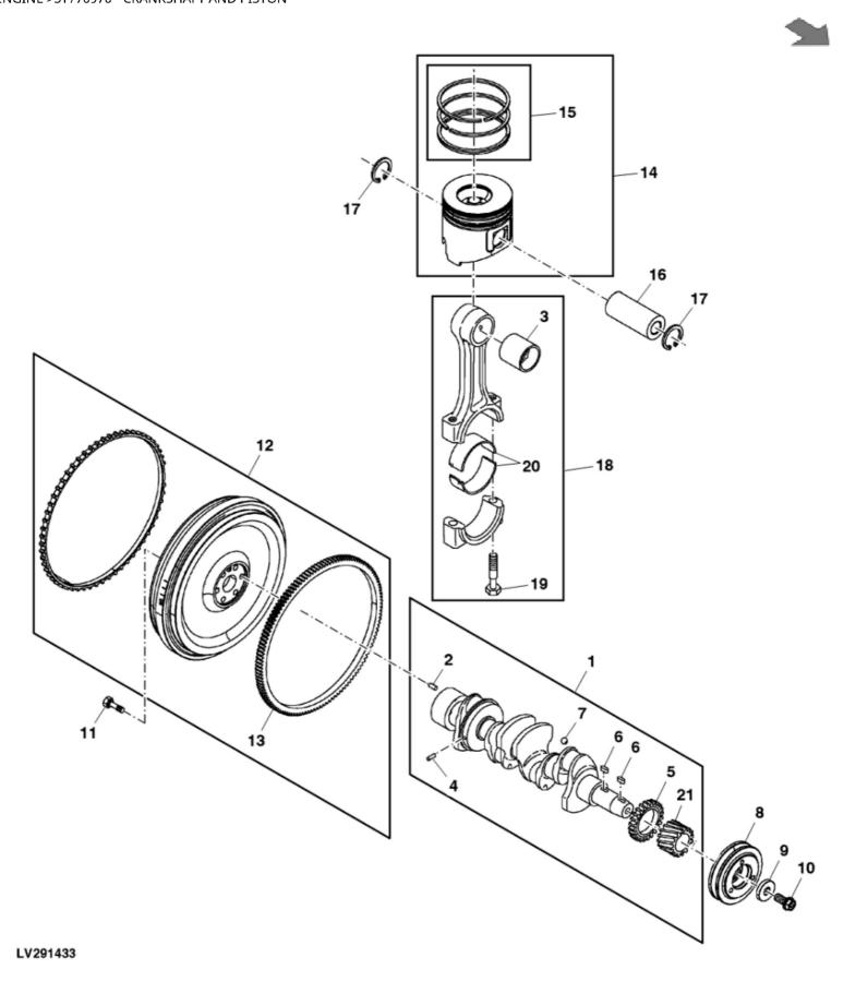
John Deere > Turf And Utility >TRACTOR, COMPACT UTILITY >4TNV86CT - TRACTOR, COMPACT UTILITY >4052M Compact Utility Tractor >20 ENGINE >ST770970 - CRANKSHAFT AND PISTON
