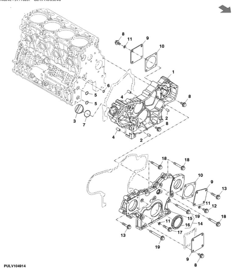
John Deere > Turf And Utility >TRACTOR, COMPACT UTILITY >4TNV86CT - TRACTOR, COMPACT UTILITY >4052M Compact Utility Tractor >20 ENGINE >ST770287 - GEAR HOUSING
