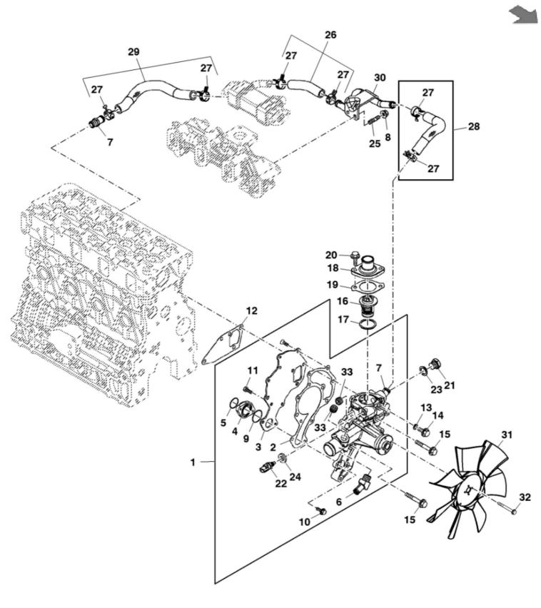
John Deere > Turf And Utility >TRACTOR, COMPACT UTILITY >4TNV86CT - TRACTOR, COMPACT UTILITY >4052M Compact Utility Tractor >20 ENGINE >ST771017 - COOLING WATER SYSTEM
