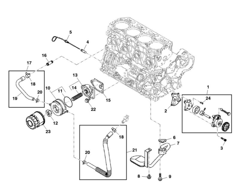
John Deere > Turf And Utility >TRACTOR, COMPACT UTILITY >4TNV86CT - TRACTOR, COMPACT UTILITY >4052M Compact Utility Tractor >20 ENGINE >ST771005 - LUBRICATION OIL SYSTEM
