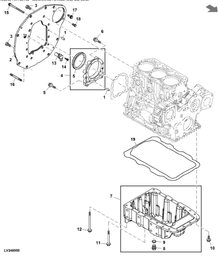
John Deere > Turf And Utility > TRACTOR, COMPACT UTILITY > 31 NV88C - TRACTOR, COMPACT UTILITY > 3039R Compact Utility Tractor > 20 ENGINE > 51768140 - MOUNTING FLANGE AND OIL SUMP
