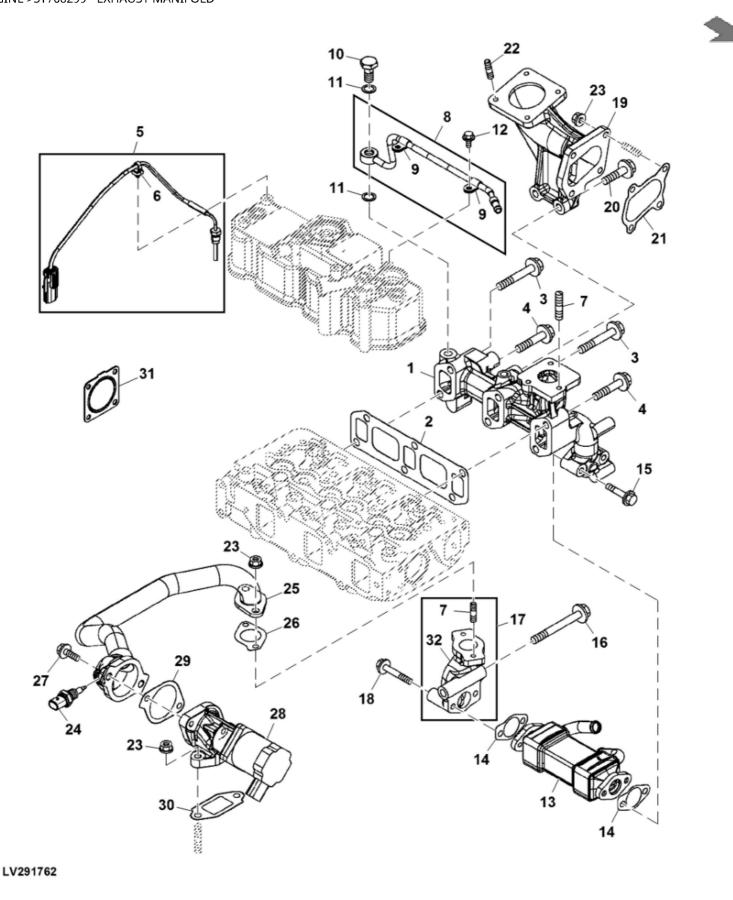
John Deere > Turf And Utility >TRACTOR, COMPACT UTILITY >3TNV88C - TRACTOR, COMPACT UTILITY >3039R Compact Utility Tractor >20 ENGINE >ST768299 - EXHAUST MANIFOLD
