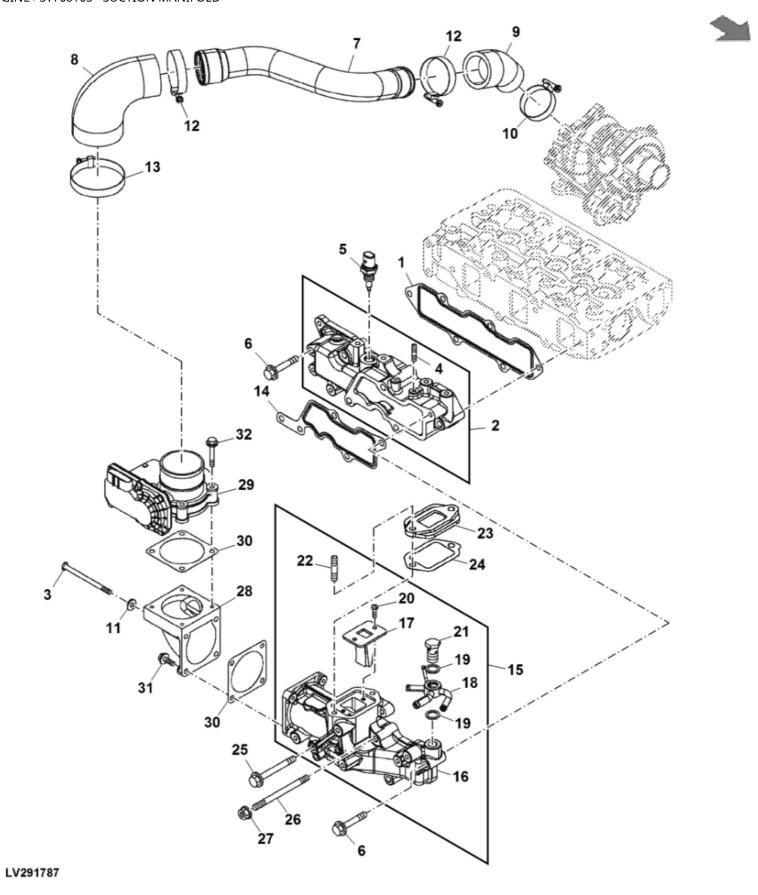
John Deere > Turf And Utility >TRACTOR, COMPACT UTILITY >31NV88C - TRACTOR, COMPACT UTILITY >3039R Compact Utility Tractor >20 ENGINE > ST768165 - SUCTION MANIFOLD
