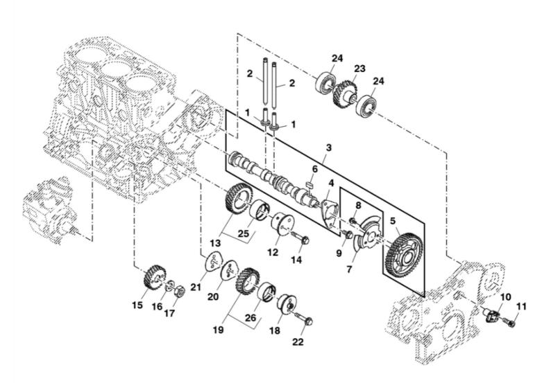
John Deere > Turf And Utility >TRACTOR, COMPACT UTILITY >3TNV88C - TRACTOR, COMPACT UTILITY >3039R Compact Utility Tractor >20 ENGINE >ST768784 - CAMSHAFT AND DRIVING GEAR
