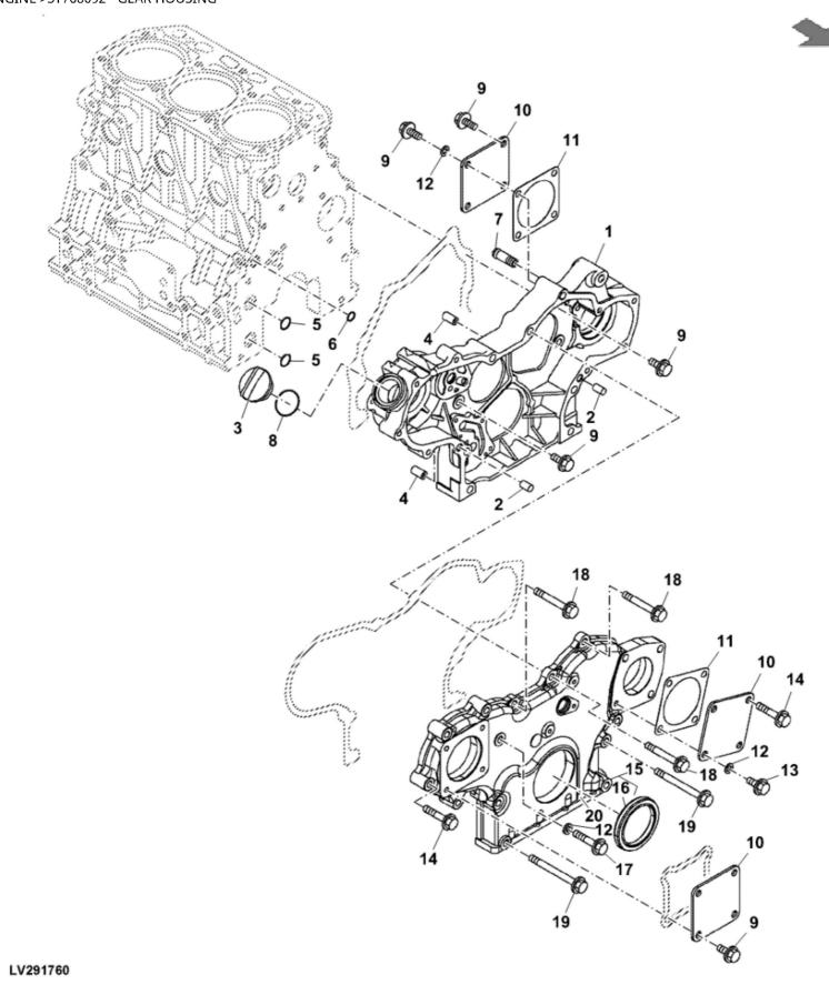
John Deere > Turf And Utility >TRACTOR, COMPACT UTILITY >3TNV88C - TRACTOR, COMPACT UTILITY >3039R Compact Utility Tractor >20 ENGINE >ST768092 - GEAR HOUSING
