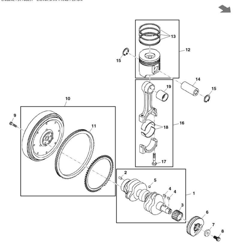
John Deere > Turf And Utility >TRACTOR, COMPACT UTILITY >3TNV88C - TRACTOR, COMPACT UTILITY >3039R Compact Utility Tractor > 20 ENGINE > 5T768897 - CRANK SHAFT AND PISTON
