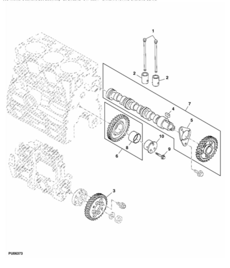
>ST745591 - CAMSHAFTS AND DRIVING GEARS
