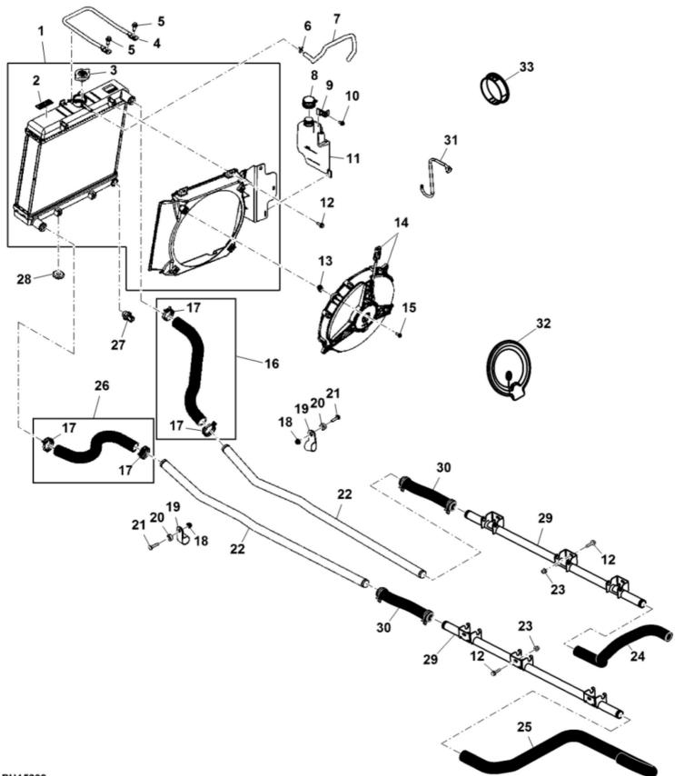
John Deere > Turf And Utility >UTILITY VEHICLE >XUV - UTILITY VEHICLE >XUV Gator Utility Vehicle 855D S4 >20 ENGINE MM17028 >ST729772 - RADIATOR
