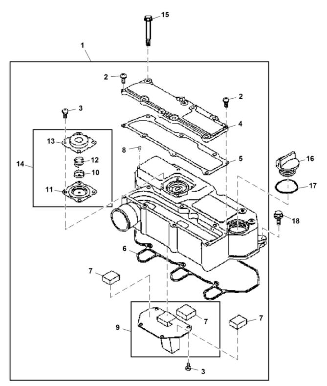
John Deere > Turf And Utility >UTILITY VEHICLE >XUV - UTILITY VEHICLE >XUV Gator Utility Vehicle 855D S4 >20 ENGINE MM17028 >ST729819 - CYLINDER HEAD COVER AND GASKETS
