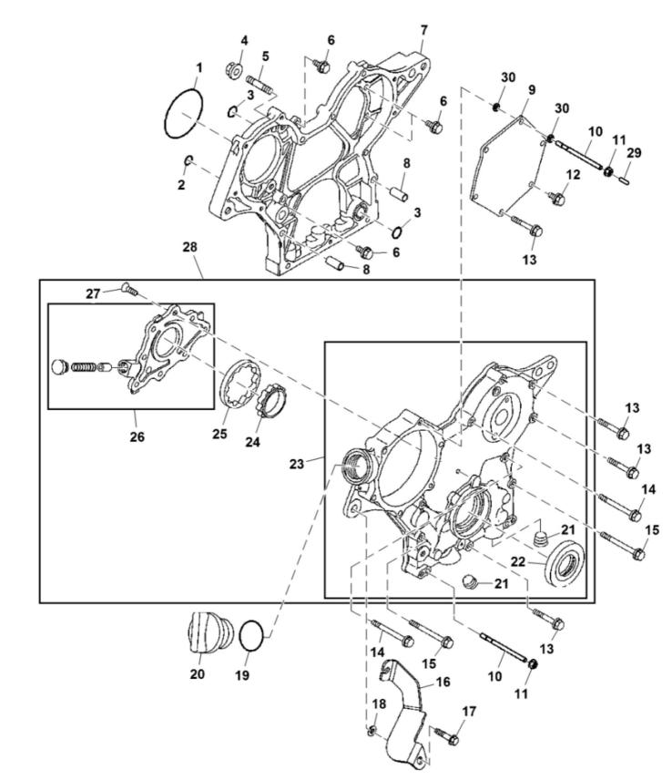
John Deere > Turf And Utility >UTILITY VEHICLE >XUV - UTILITY VEHICLE >XUV Gator Utility Vehicle 855D S4 >20 ENGINE MM17028 >ST729823 - GEARCASE AND OIL PUMP
