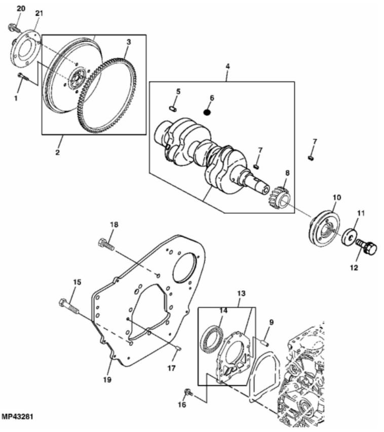
John Deere > Turf And Utility >UTILITY VEHICLE >XUV - UTILITY VEHICLE >XUV Gator Utility Vehicle 855D S4 >20 ENGINE MM17028 >ST729817 - CRANKSHAFT, FLYWHEEL AND MOUNTING FLANGE
