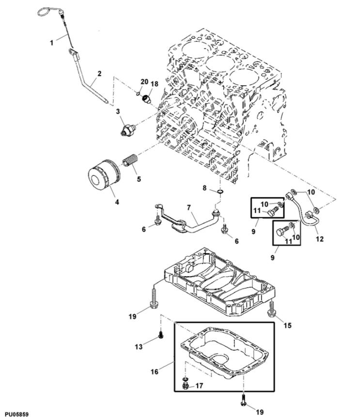
John Deere > Turf And Utility >UTILITY VEHICLE >XUV - UTILITY VEHICLE >XUV Gator Utility Vehicle 855D S4 >20 ENGINE MM17028 >ST729822 - ENGINE OIL FILTER AND OIL SUMP
