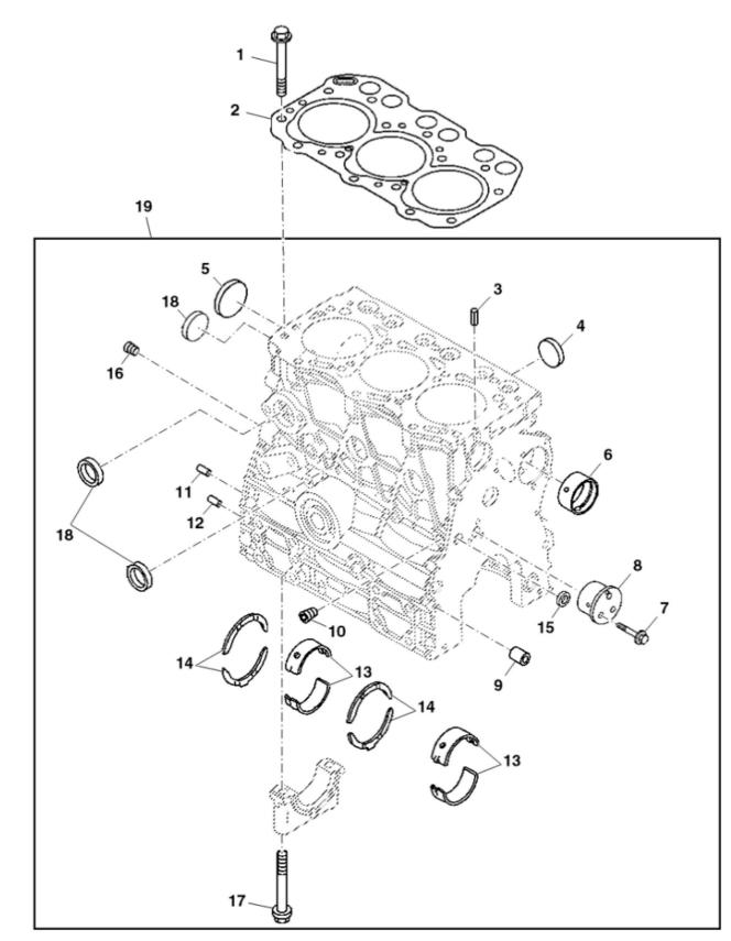
John Deere > Turf And Utility >UTILITY VEHICLE >XUV - UTILITY VEHICLE >XUV Gator Utility Vehicle 855D S4 >20 ENGINE MM17028 >ST729815 - CYLINDER BLOCK
