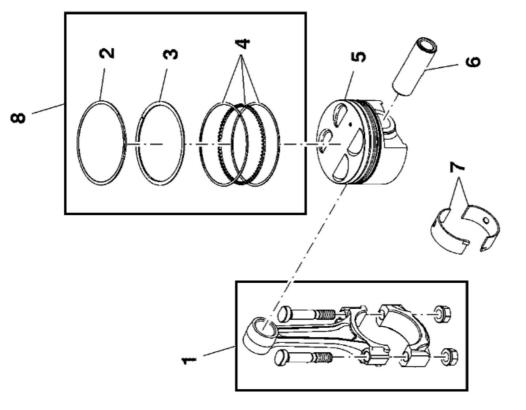
John Deere > Turf And Utility > UTILITY VEHICLE > XUV - UTILITY VEHICLE > XUV Gator Utility Vehicle 825I S4 > 20 ENGINE MM17029 > ST729774 - CONNECTING ROD AND PISTON
