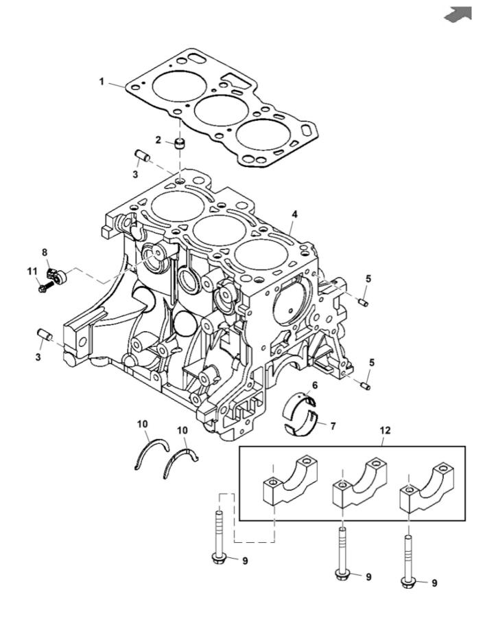
John Deere > Turf And Utility > UTILITY VEHICLE > XUV - UTILITY VEHICLE > XUV Gator Utility Vehicle 825I S4 > 20 ENGINE MM17029 > ST729773 - CYLINDER BLOCK
