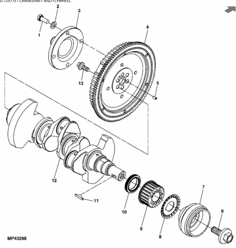
John Deere > Turf And Utility > UTILITY VEHICLE > XUV - UTILITY VEHICLE > XUV Gator Utility Vehicle 825I S4 > 20 ENGINE MM17029 > ST729775 - CRANKSHAFT AND FLYWHEEL
