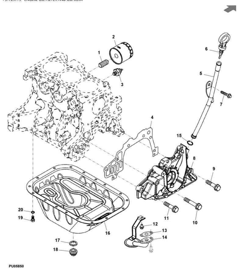
John Deere > Turf And Utility > UTILITY VEHICLE > XUV - UTILITY VEHICLE > XUV Gator Utility Vehicle 825I S4 > 20 ENGINE MM17029 > ST729779 - ENGINE OIL FILTER AND OIL SUMP
