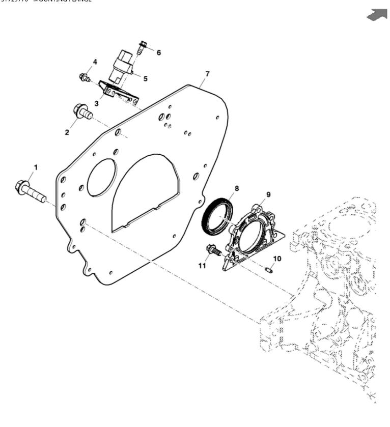
John Deere > Turf And Utility > UTILITY VEHICLE > XUV - UTILITY VEHICLE > XUV Gator Utility Vehicle 825I S4 > 20 ENGINE MM17029 > ST729776 - MOUNTING FLANGE
