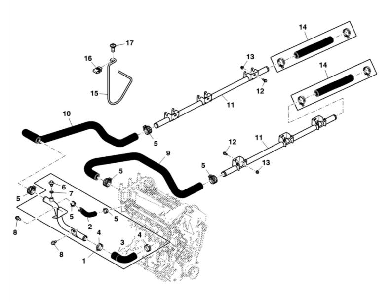
John Deere > Turf And Utility > UTILITY VEHICLE > XUV - UTILITY VEHICLE > XUV Gator Utility Vehicle 825I S4 > 20 ENGINE MM17029 > ST786736 - COOLANT LINES (080001 - )
