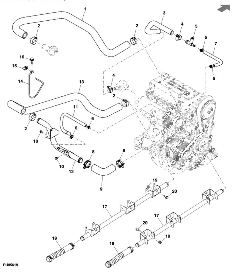
John Deere > Turf And Utility > UTILITY VEHICLE > XUV - UTILITY VEHICLE > XUV Gator Utility Vehicle 825I S4 > 20 ENGINE MM17029 > ST729783 - COOLANT LINES (-080000)
