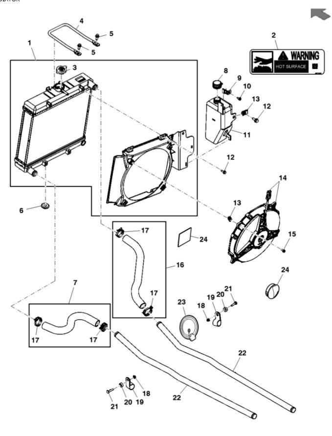
John Deere > Turf And Utility > UTILITY VEHICLE > XUV - UTILITY VEHICLE > XUV Gator Utility Vehicle 825I S4 > 20 ENGINE MM17029 > ST729782 - RADIATOR
