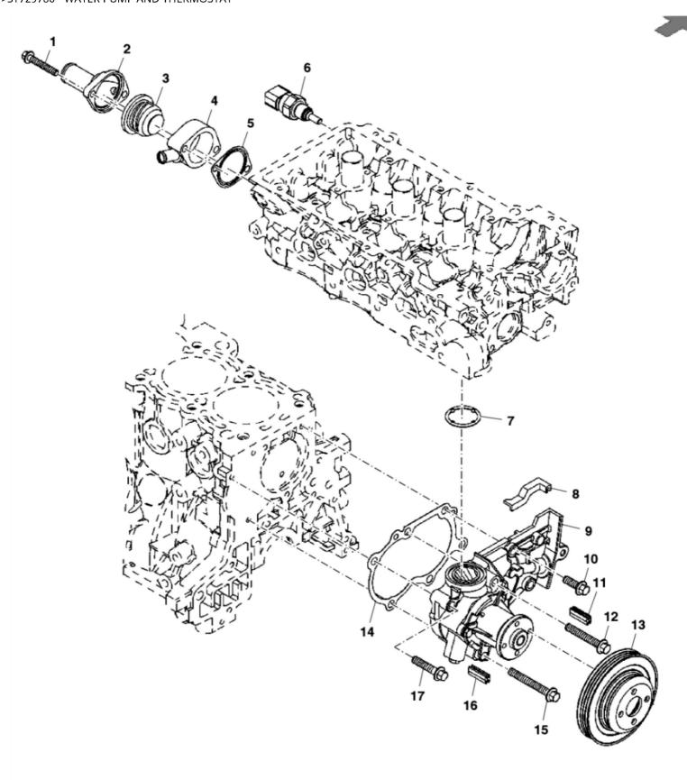
John Deere > Turf And Utility > UTILITY VEHICLE > XUV - UTILITY VEHICLE > XUV Gator Utility Vehicle 825I S4 > 20 ENGINE MM17029 > ST729780 - WATER PUMP AND THERMOSTAT
