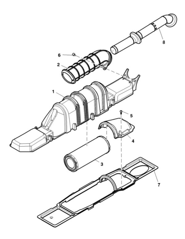
John Deere > Turf And Utility > UTILITY VEHICLE > XUV550 - UTILITY VEHICLE > XUV550 Gator Utility Vehicle > 30 FUEL AND AIR > ST584160 - AIR CLEANER
