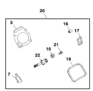
John Deere > Turf And Utility > UTILITY VEHICLE > XUV550 - UTILITY VEHICLE > XUV550 Gator Utility Vehicle > 20 ENGINE MM17462 > ST584192 - ENGINE GASKET KIT
