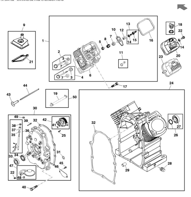
John Deere > Turf And Utility > UTILITY VEHICLE > XUV550 - UTILITY VEHICLE > XUV550 Gator Utility Vehicle > 20 ENGINE MM17462 > ST584162 - CRANKCASE AND CYLINDER HEAD
