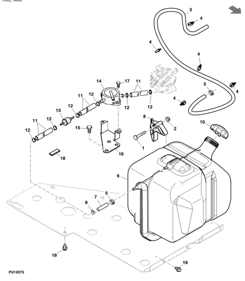
John Deere > Turf And Utility > UTILITY VEHICLE > XUV550 - UTILITY VEHICLE > XUV550 Gator Utility Vehicle > 30 FUEL AND AIR > ST593936 - FUEL TANK
