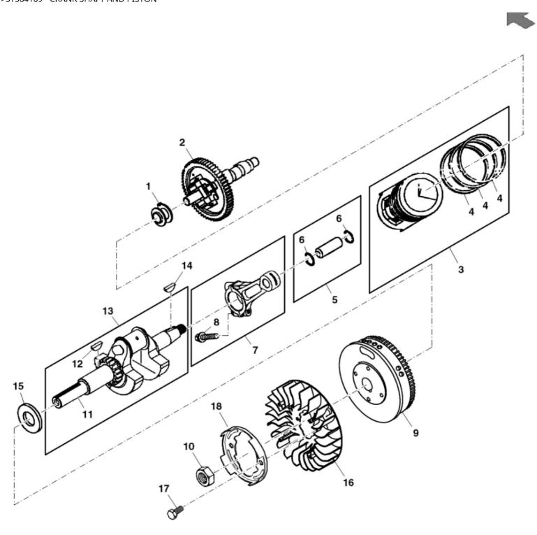
John Deere > Turf And Utility > UTILITY VEHICLE > XUV550 - UTILITY VEHICLE > XUV550 Gator Utility Vehicle > 20 ENGINE MM17462 > ST584169 - CRANK SHAFT AND PISTON
