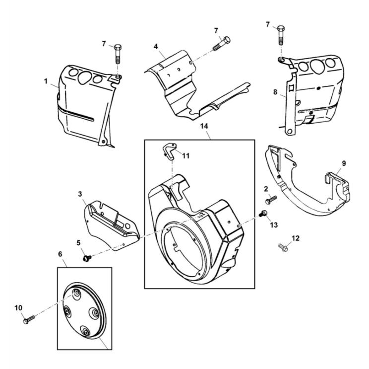
John Deere > Turf And Utility > UTILITY VEHICLE > XUV550 - UTILITY VEHICLE > XUV550 Gator Utility Vehicle > 20 ENGINE MM17462 > ST584184 - ENGINE BLOWER HOUSING
