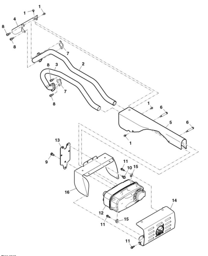
John Deere > Turf And Utility > UTILITY VEHICLE > XUV550 - UTILITY VEHICLE > XUV550 Gator Utility Vehicle > 30 FUEL AND AIR > ST563706 - MUFFLER
