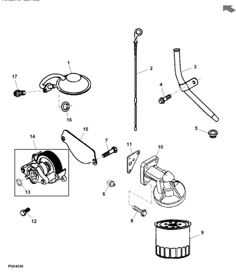
John Deere > Turf And Utility > UTILITY VEHICLE > XUV550 - UTILITY VEHICLE > XUV550 Gator Utility Vehicle > 20 ENGINE MM17462 > ST584176 - OIL PUMP
