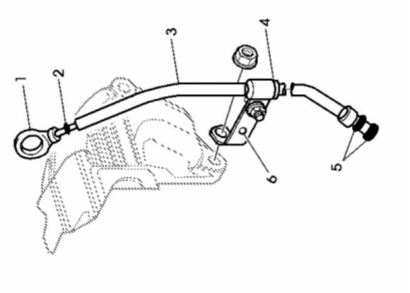
John Deere > Turf And Utility > TRACTOR, COMPACT UTILITY > 100F - TRACTOR, COMPACT UTILITY > 100F Orchard and Vineyard Tractor > 20 ENGINE TRACTOR > ST321662 - ENGINE OIL DIPSTICK
