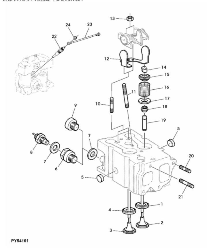
John Deere > Turf And Utility >TRACTOR, COMPACT UTILITY >100F - TRACTOR, COMPACT UTILITY >100F Orchard and Vineyard Tractor >20 ENGINE TRACTOR >ST380323 - VALVE/VALVE SEAT
