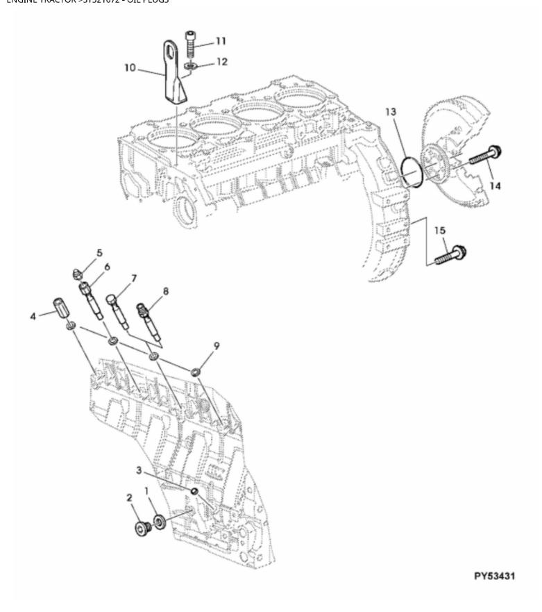
John Deere > Turf And Utility >TRACTOR, COMPACT UTILITY > 100F - TRACTOR, COMPACT UTILITY > 100F Orchard and Vineyard Tractor > 20 ENGINE TRACTOR > ST321672 - OIL PLUGS
