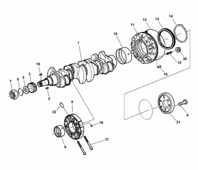
John Deere > Turf And Utility >TRACTOR, COMPACT UTILITY > 100F - TRACTOR, COMPACT UTILITY > 100F Orchard and Vineyard Tractor > 20 ENGINE TRACTOR > ST321677 - CRANK SHAFT/BEARINGS
