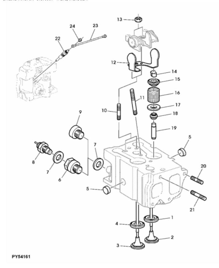
John Deere > Turf And Utility >TRACTOR, COMPACT UTILITY >85F - TRACTOR, COMPACT UTILITY >85F Orchard and Vineyard Tractor >20 ENGINE TRACTOR >ST379981 - VALVE/VALVE SEAT
