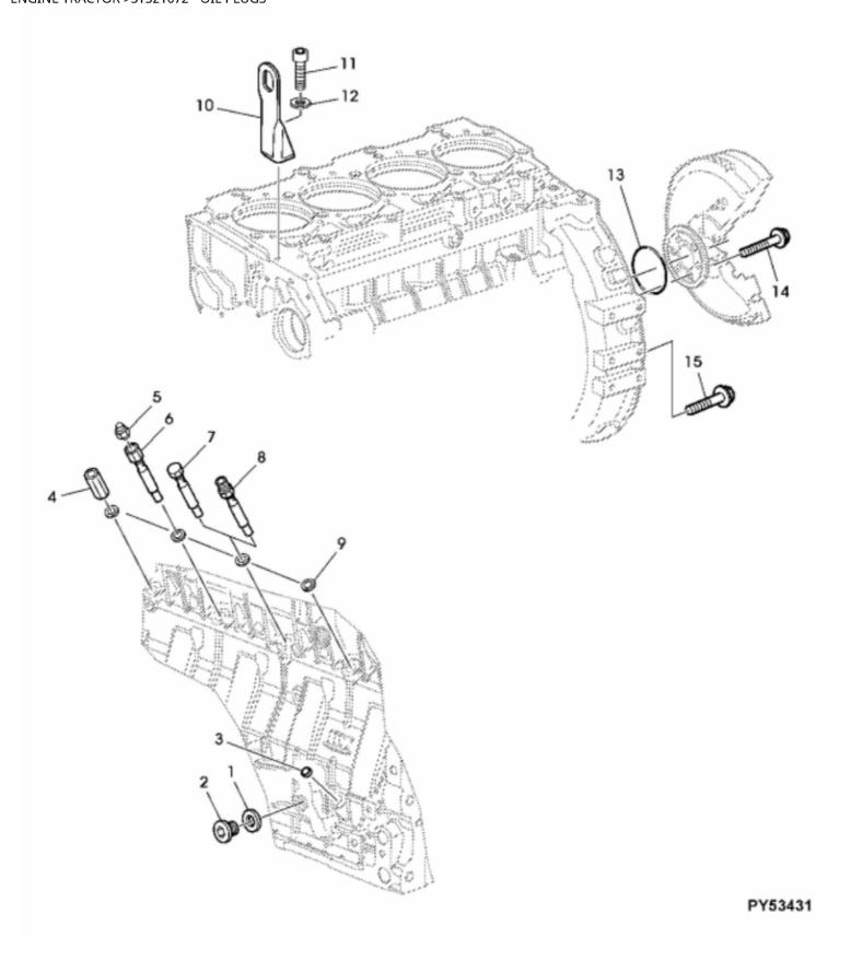
John Deere > Turf And Utility >TRACTOR, COMPACT UTILITY >85F - TRACTOR, COMPACT UTILITY >85F Orchard and Vineyard Tractor >20 ENGINE TRACTOR >ST321672 - OIL PLUGS
