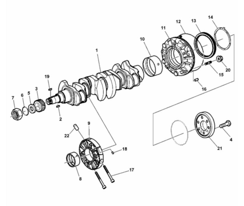
John Deere > Turf And Utility >TRACTOR, COMPACT UTILITY >85F - TRACTOR, COMPACT UTILITY >85F Orchard and Vineyard Tractor >20 ENGINE TRACTOR >ST379976 - CRANK SHAFT/BEARINGS
