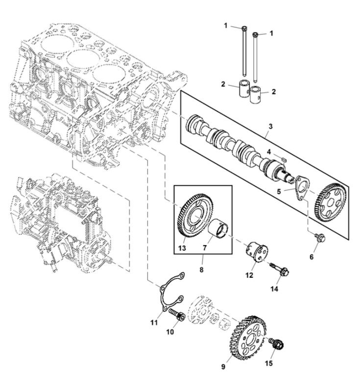
CAMSHAFTS AND DRIVING GEARS
