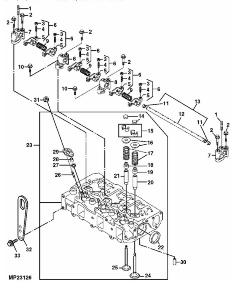
John Deere > Turf And Utility >TRACTOR, COMPACT UTILITY > 4400 - TRACTOR, COMPACT UTILITY > 4400 Compact Utility Tractors > 20 ENGINE (4400) > 5T632334 - CYLINDER HEAD, VALVES AND ROCKER ARMS
