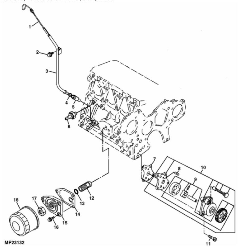
John Deere > Turf And Utility > TRACTOR, COMPACT UTILITY > 4400 - TRACTOR, COMPACT UTILITY > 4400 Compact Utility Tractors > 20 ENGINE (4400) > 5T632341 - ENGINE OIL PUMP, FILTER / DIPSTICK
