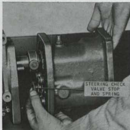
Fig. 12—Remove steering check valve stop and spring as unit is separated.
