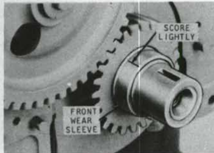
Fig. 18—Score oil seal wear sleeve as shown using blunt chisel, then pry from shaft when renewal is indicated.
