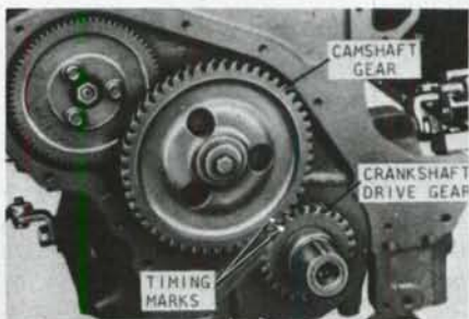
Fig. 19—Timing gears with cover removed, showing timing marks on turbocharged model. Other models are similar.
