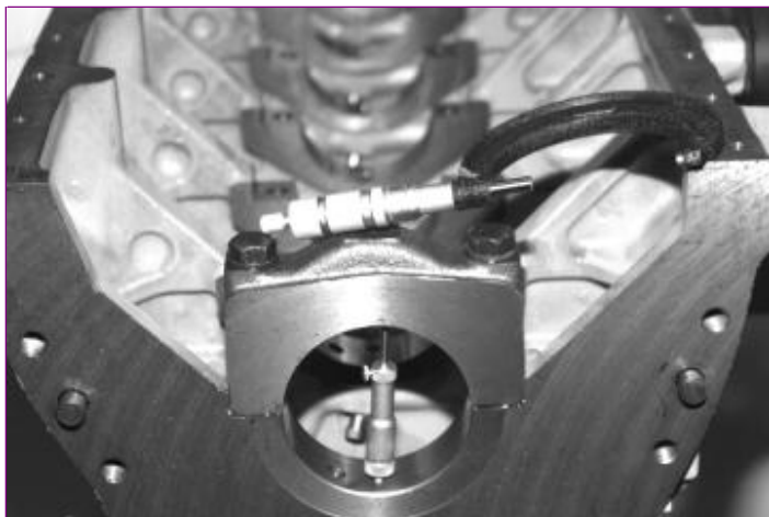
RG7537-UN: Measuring Assembled Main Bearing Cap ID
