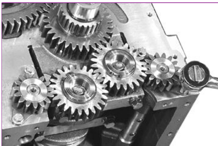
RG13039-UN: Balancer Shaft Removal
