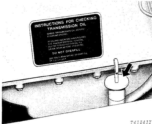
Fig. 12-Transmission-Hydraulic System Filler Cap and Dipstick
