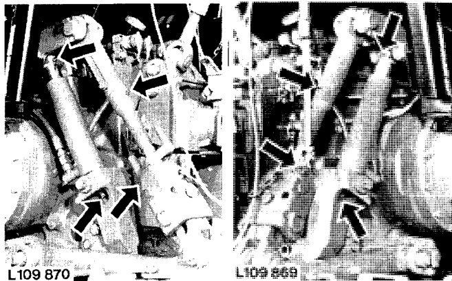
Fig. 31 – Grease Fittings of Lift Links and Extra Cylinder (Tractors with Increased Lifting Capacity)
