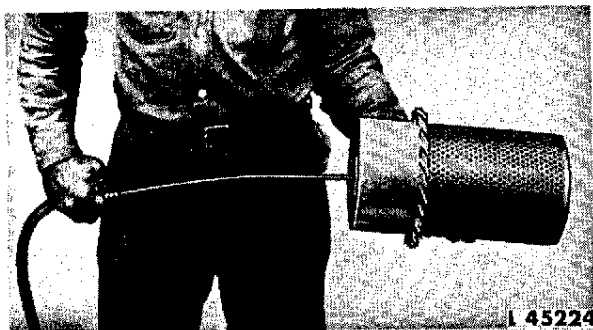
Fig. 2 - Cleaning Air Cleaner Element by Means of Compressed Air
