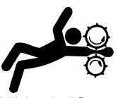
Tie long hair behind your head. Do not wear a necktie, scarf, loose clothing, or necklace when you work near machine tools or moving parts. If these items were to get caught, severe injury could result.
