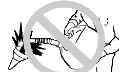
NO STATIC ELECTRIC DISCHARGE
