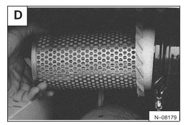
Remove the filter element [D].
