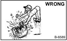
Lead-acid batteries produce flammable and explosive gases. Keep arcs, sparks, flames and lighted tobacco away from
