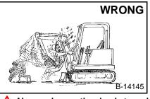
Always lower the bucket and blade to the ground before doing any maintenance. Never modify equipment or add
