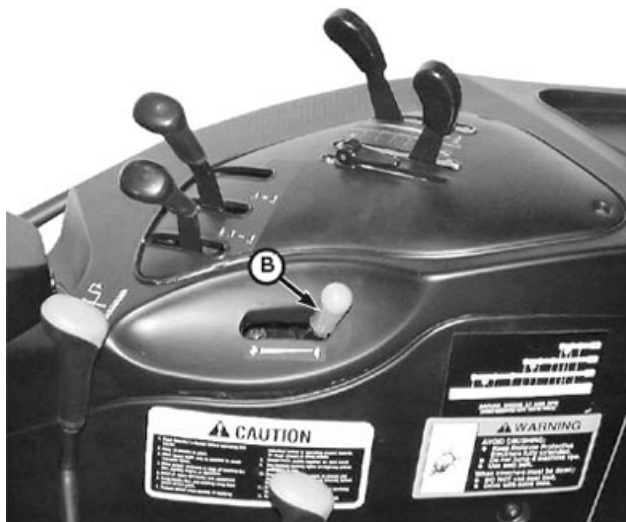
A—Throttle Lever (Straddle Mount Tractor) B—Throttle Lever (Isolated Open Operator Station and Cab Tractor)
